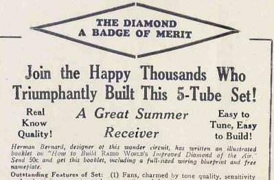
Outstanding Features of Set: (1) Fans, charmed by tone quality, sensitivity and selectivity, report speaker reception of far-distant stations with great volume. (2) A 2-tube earphone set, a 5-tube speaker set, and a separate 3-stage (3) No rheostats are used. (4) The set is inexpensive to construct and maintain. (5) The set works from outdoor aerial or loop, hence no aerial problems present themselves, in city or country
