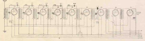
A WELL-BALANCED 9-tube receiver. Six stages of tuned radio frequency amplification, a non-regenerative detector and two stages of transformer coupled AF amplification are used. The first five stages of RF amplification are neutralized. The variable condenser may be ganged on one shaft, making it one-control.
