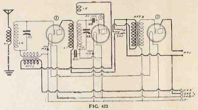
The circuit diagram of the 3-tube reflex, desired by James Klein.
