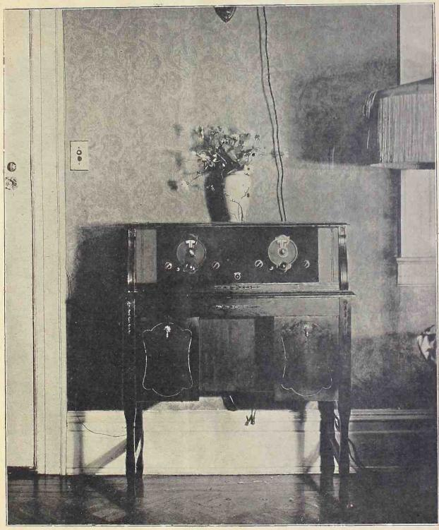
FIG. 1 The 6-tube Victoreen Super-Heterodyne in a console that houses also the A and B eliminators.
