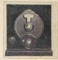
CLOSEUP of the National velvet vernier, variable ratio illuminated dial. Two of this type are used in the 1927 Victoreen. A switch at low-er left turns on or off the small bulb used for illuminating the scale.
