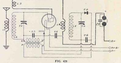
The electrical diagram of the 1-tube reflex using a crystal as a detector.
