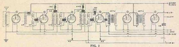
The circuit diagram of the Alden-Somerbridge balanced receiver.
