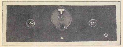
FIG. 3 The panel view of the one control set. The switch is mounted with lamp horizontal.
