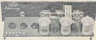
Rear view of the Welty Etherway, chassis model. This is a 5-tube laboratory-constructed receiver.
