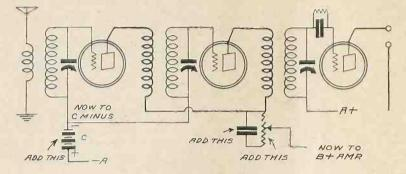
FIG. 1 The essential details of the wiring of a tuned radio frequency receiver, up to and including the detector, as shown is the top diagram, to illustrate leads that will be changed so as to embody the Bernard system of neutralization. The changes to be made are illustrated in the lower diagram. In most sets the audio C battery will be used, so that only the variable high resistance and the bypass condenser need be added to the set.
