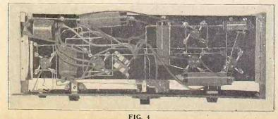
All the wiring is done underneath the subpanel. Note how bracket at left is cut.
