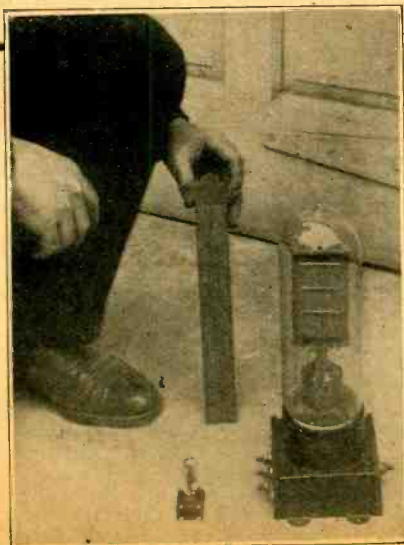
(Herbert Photos, Inc.) THE comparative sizes of the small peanut dry-cell and the gigantic and powerful 1500 watt tube are shown.
