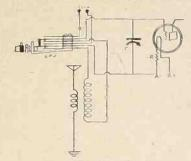
FIG. 455 The circuit diagram, illustrating how to hookup a Carter No. 6 jack switch, for loop-antenna switching.
