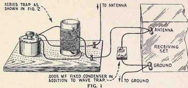
Picture diagram of a series wave trap, used for eliminating interference. Note the .0005 mfd. fixed condenser across the antenna and ground posts of the set
