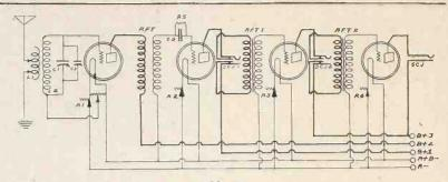
FIG. 454 The circuit diagram of the 4-tube receiver using untuned detector and a tuned detector stage.
