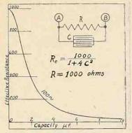
FIG. 2 The change in effective resistance with values of Co from 0 to 10 mfd.
