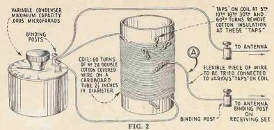
How a parallel wave trap is connected.
