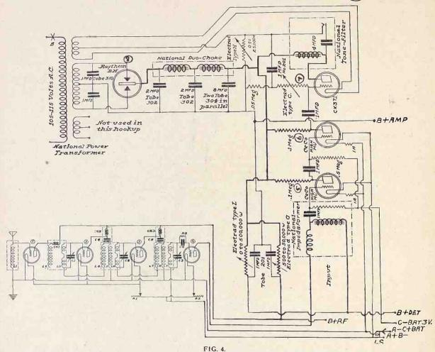
How to wire up an Alden-Somerbridge Circuit (lower left) to work in conjunction with the Lynch Lamp Socket Amplifier. Eight tubes are required, including the Raytheon type BH (upper left). The Alden-Somerbridge Circuit is a balanced radio receiver, without audio. The Lynch Lamp Socket Amplifier consists of an eliminator of all B batteries, and A eliminator and C eliminator for the final audio tube, and a splendid tone quality 3-stage audio amplifier.
