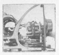
MOST FOLK use some type of flux when soldering. This, if not properly handled, smears all over the joint, causing a high resistance, resulting in its attendant losses. However, most trouble is encountered when soldering the terminals of the jack, due to the odd position of the prongs. With the aid of a small paint brush, this excess paste may be taken off. First immerse the brush in alcohol. Most of the paste will be found between the in-
