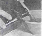
IN making a storage battery solution, always add the acid (sulphuric, H2SO4), slowly to the water, and not the water to the acid. If the opposite method is employed, a boiling and sputtering of the solution will take place. After each few drops of the acid are added in the correct fashion. stir carefully.
