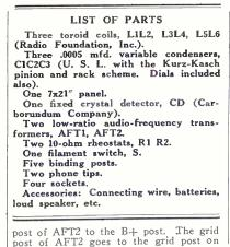
socket 4. The F— post goes to the F— post on socket 4. This in turn goes to the resistance wire of the rheostat R2. Connect the F+ posts together. The plate post of the last socket goes to one phone tip. The other phone tip goes to the B+ post. One terminal of the switch S, goes to the arms of both rheo-stats, R1 and 2. The other terminal of this switch goes to the A+B— post. When following the diagram. reverse the When following the diagram, reverse the A battery leads.
