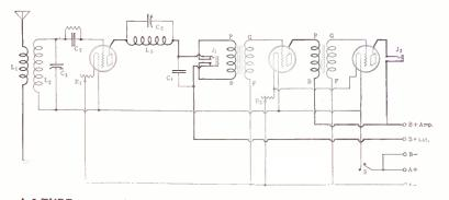
A 3-TUBE regenerative receiver with a variable condenser, C2, having a capacity of .0005 mfd. tuning the plate. R1 is a 10-ohm rheostat, while R2 is a 6-ohm rheostat.
