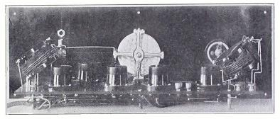
THE REAR VIEW (Fig. 4) shows the coils mounted at an angle of about 57 degrees, simply as an extra safeguard against stray coupling. The aerial and ground posts are at right. The two cup-like objects a few inches to the left of these posts are the phone tip jacks. The speaker cord tips are inserted here. The sockets are, left to right: first AF, detector, second AF, third AF and RF, i.e., as designated in Fig. 1, they are 3, 2, 4, 5 and 1.
