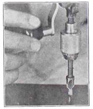
INSTEAD of taking the drill out of the bit to insert a countersink you and may use a combination drill countersink. After the drill has panel the countersink pierced the functions.
