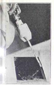
PHOTOGRAPH shows how to hole in a panel, without having il slip oll over the panel, thereby cracing it and delaying the work. Lace piece of wood snug up against ince where the hole is to be rill. Tighten down with a vice. he you can drill the hole without ny ar of the drill slipping, as it y rest up against the board.
