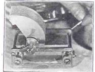
WHEN you test a variable condenser for a complete circuit a faint click may be heard, due to the charge and discharge of the condenser. Should you hear a loud click there is a short circuit in the condenser, that is, plates are touching each other.
