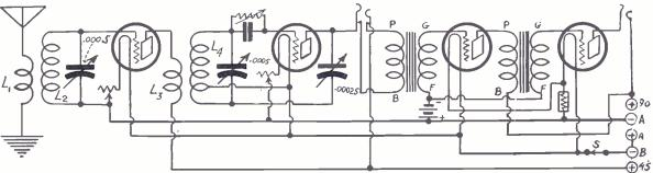
FIG. 1 shows the circuit diagram of the 4-tube DX Symphony. This set uses one stage of tuned radio-frequency amplification, a detector regenerated by the Hartley system, and two stages of audio-frequency amplification, employing transformers. As for the switching plan consult text.
