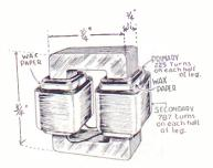
HOW an AC transformer with an output of 340 volts is wound is shown above. No. 22 SCE wire is used to wind the primary and No. 30 SCE is used to wind the secondary.
