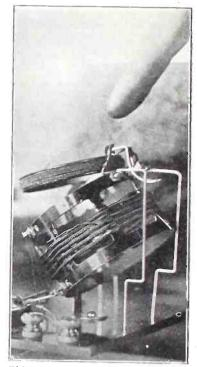
FIG. 7, the adjustable primary. This differs from a variable primary in that the adjustment, once made, is left that way.
