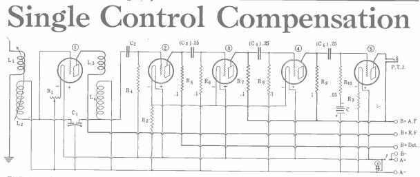
THE circuit diagram (Fig. 1) of the 1-dial receiver, with a separate B-plus lead for the RF amplifier tube, as this voltage must be just right. The primary is adjustable, as distinguished from a variable primary. A pilot lamp is used (lower right).
