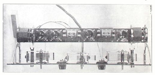
Wiring Is Simple and Even a Novice May Construct The Receiver and Obtain Fine Results — Coils Should be of the Type Suitable for Tuning With Straight-line Frequency Condensers
