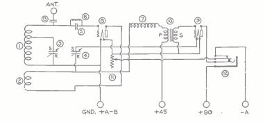
The constants of this circuit follow, with the apparatus used at 2APJ cited: (1)—Secondary coil, 9 turns wound on a 3/2'' quartzite form. A tap is taken 3 turns from the grid side of the coil. The condenser (3) is placed across the remulting 6 turns for remaining 6 turns. (2)—Tickler coil, 5 turns wound on the
