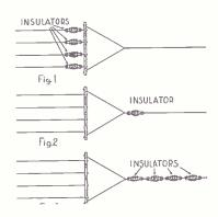
placed at the extreme end of the antenna, as in Fig. 2, for then the total resistance would be 40 ohms. If the four insulators were connected in tandem as in Fig. 3, the total resistance would be 160 ohms or sixteen times as much insulation as with the arrangement in Fig. 1.
