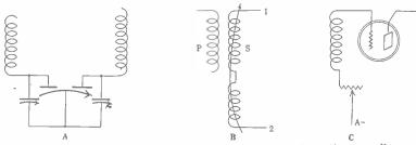
FIG. 2—A variable primary may be used as a balancer (Fig. 1) or small extra condensers may be used ("A"), or inductive variation in a conductively coupled secondary may be employed ("B") or the inductance of a rheostat may be utilized (a bad method).
