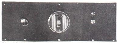
THE PANEL view of the 5-tube receiver diagrammed on the opposite page. The knob at left is the RF rheostat, R1 in Fig. 1. The switch at right lights or unlights all five tubes. The aperture above it is an opaque marcon window, illuminated by a pilot light when the set is "on." In center is the single tuning control, a dial that makes any condenser that is not straight-line frequency tune just as if the condenser were such. (Fig. 3.)
