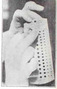
With the above chart, which is called a drill and Wire Gauge Chart for Machine Screw Taps, you can learn the standard number and size in decithe standard number and size in deci-mals of an inch, of all types of ma-chine screws. This enables you to know what size hole to drill in the panel. Besides finding out the size of screws, the diameters of shafts, of condensers, couplers, etc., may also be ascertained by inserting the shaft into the holes.
