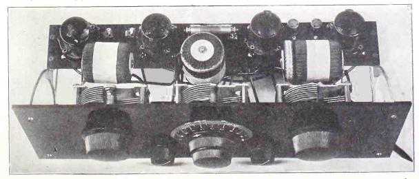
TOP VIEW. The tuning dial is vernier, while the compensating knobs adjust the first RF and detector input condensers for synchronized tuning. The toroids are mounted on the socket shelf behind the U. S. L. condensers.
