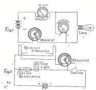
T HE incorporation of a pilot light for the purpose of illuminating the tuning dial, or as an indication when the tubes of the set are "on," is an innovation acquiring increased popularity each day, among both constructively inclined radio fans and radio receiver manufacturers. But even such a simple item has its complication. This is the selection of the lamp with respect to the filament voltage and current constants.
