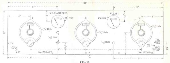
simple to operate. However, if you know anything about radio you must appreciate that independent dial settings are more efficient than unicontrol. It is common knowledge that circuits can be made electrically alike, but such circuits will not stay that way very long. Efficiency, being the paramount factor in this set, necessitated three dials.
