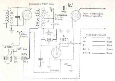
FIG. 1. The 2-to-5 meg. Leak goes from first detector grid to A+.
