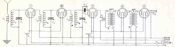
wound to constitute the primaries and 65 turns wound to constitute the secondaries. There is a  $\frac{1}{4}$ " space left between wind-The tap is made at the 10th turn, on ings. secondary of the second RFT.
