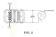
the second coil, and there is no direct connection other than via the magnetic field. The number of lines of force which
