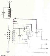
FIG. 1, wiring diagram of the receiver in schematic form, showing grid re-turn to negative A, which works well on only a very few types of tubes, not including the 99.
