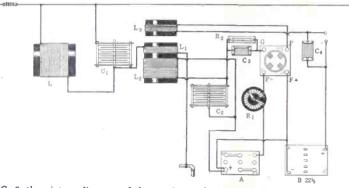
FIG. 2, the picture diagram of the receiver, which will be of material assistance to movices who desire to construct the voluminous DX set described in the accompanying article.
