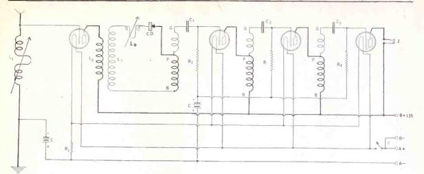
FIG. 255 showing the electrical diagram of the receiver Mr. Greenstein requested.
