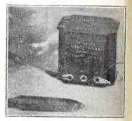
WHEN soldering to a transformer post (which itself is soldered to a primary or secondary lead) quickly cool the joint with water. A brush serves the purpose. Thus you do not melt the soldered winding terminal off the post. (Hayden).
