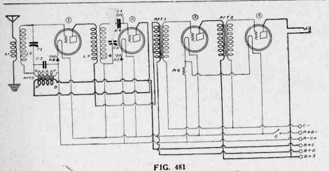
The circuit diagram of the 4-tube reflex
