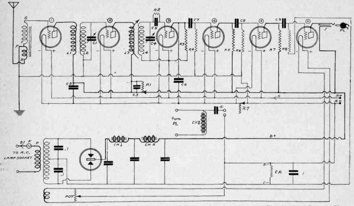
THOSE desiring to build the Bernard receiver to operate 5-volt tubes without batteries may follow the above diagram. The unmarked filter condensers are, left to right, 2, 2 and 4 mfd., 600-volt test. Tube 6 is a -71 power bulb. The A eliminator may be a Radi-A or a Davey. The line current must be AC. CR is a 750 ohm Ward Leonard. See December 4 issue for other constants.
