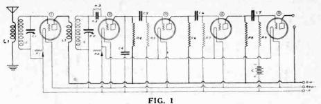
Design of a circuit using resistance coupled audio frequency amplifications throughout. Tubes 3 and 4 should be high mu, while tube 5 should be a power tube. If the highest B voltage used is 90 a common lead, may be employed, but 90 is an inefficient voltage for resistance coupling.
