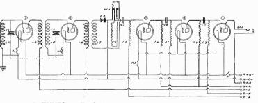
A TUNED radio frequency set with crystal detector.
