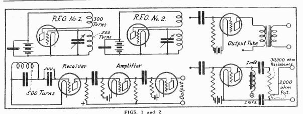
The fundamentals of the hookup for the beat note audio oscillator, and methods of effecting output.
