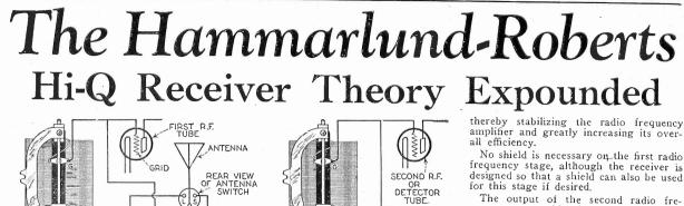
The output of the second radio frequency stage, which is a highly amplified copy of the original signal picked up by the antenna, is then fed to the non-regenerative detector, where it is demodulated or converted into audible frequencies. These audio currents, or electric sound waves, are then further increased in strength by the two stages of transformer coupled audio frequency amplification and passed on to the loudspeaker.
