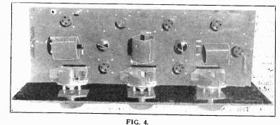
The top view of the receiver. Note the Benjamin coils, condensers and sockets.
