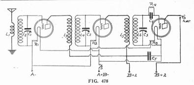
The circuit diagram of the tuned RF and detector unit requested by Thomas ' Rougher
