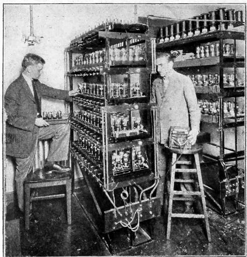
(Underwood & Underwood) VACUUM TUBES being tested for their duration of life in a test rack. Each tube is tested with precision instruments.
