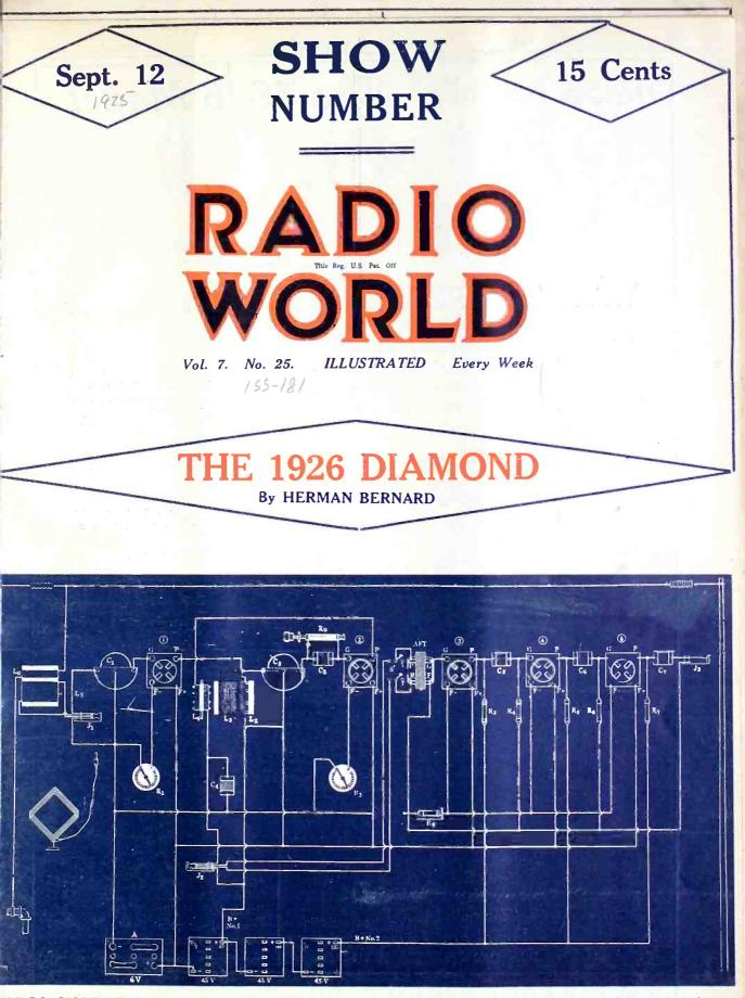
ADIO WORLD'S most popular circuit, The Diamond of the Air, shown in blueprint form. his is the 1926 model, embodying the Bernard audio amplifier. See page 5 for article on construction of this receiver.
