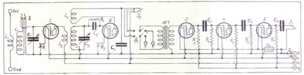
FIG. 1, the wiring diagram of the 1926 Model Diamond of the Air. The improvement is exclusively in the audio circuit and the greater possibilities of using it. The double-pole double-throw switch enables use of the audio hook-up in conjunction with any other set or detector test circuit. The AF consists of one transformer stage and two resistance steps. A novelty exists in the speaker connections, one speaker tip going to A—, the other to one side of a large condenser. This is a quality asset.
