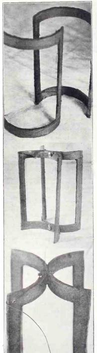
FIG. 6 (top), the two pieces after the tubing has been cut. Fig. 7, reverse the halves and fasten together. Fig. 8, secure the magnet wire (No. 22 DSC) as shown.
