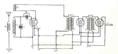
FIG. 200, showing the electrical diagram of a 3-tube set. The constants for the coil are the same as in the coil of Fig. 199. C1 is a .0005 mfd. variable condenser. C2 is the .00025 grid condenser. R1 is a 2 megohm grid leak resistance. A 6-ohm resistance is used to control the filaments of the UV201A tubes. The new UX tubes may be used here also. AFT 1 and 2 are both of the low ratio type.
