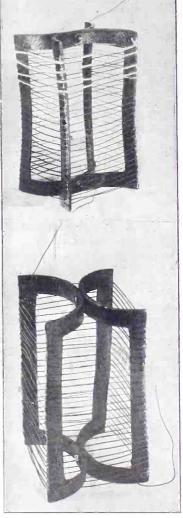
r 1G. 9 (top) shows an RF transformer, 4 turns No. 18 DCC wire for primary, 25 turns No. 22 DSC wire for secondary. Fig. 10 is an impedance coil. (Hayden Photos)
