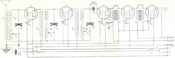
FIG. 3, showing the electrical wiring of the 5-Tube Inductively-coupled receiver.
