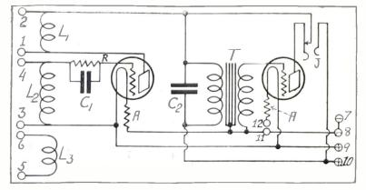
FIG. 1, the wiring of Anderson's oscillating wavemeter.
