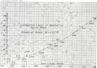
FIG. 3, a calibration chart of Anderson's oscillating wavemeter.
