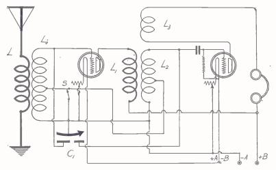
FIG. 5, a double condenser, C1, used to tune two stages at once, the switch S tapping each secondary at the same relative point.
