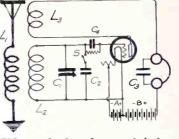
FIG. 2, a fixed condenser switched on for parallel connection with C1.
