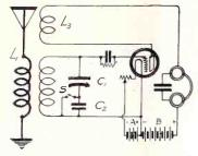
FIG. 1, a fixed condenser in series with C1, a switch S being used for cutting out this condenser by the short-circuiting method.
