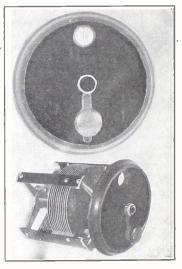
FIG. 9 (top), the front of the dial, with the dial reading visible through the window. The slot is in plain view, with the travelling dial knob in it. The center circle is a decorative knob behind which is a bushing with thread and screw for engaging the condenser shaft.
