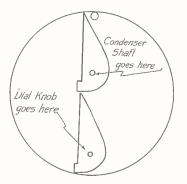
FIG. 7, the fundamental idea of a straight-line frequency dial.
