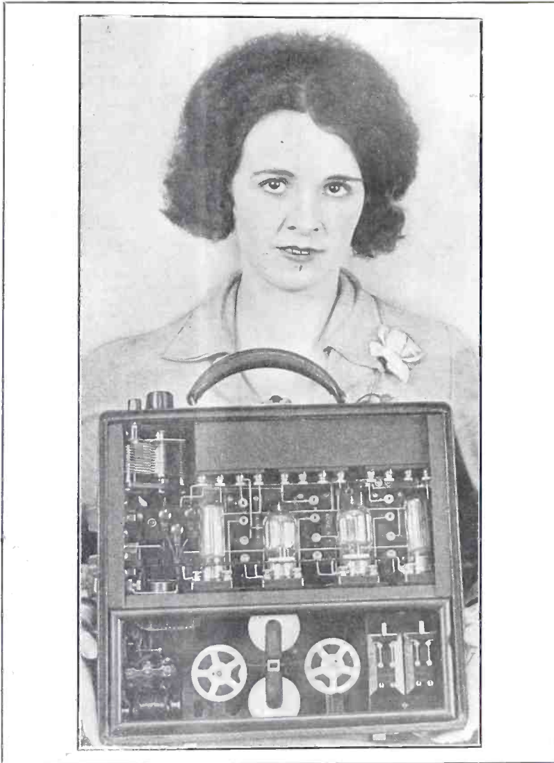
THIS 4-tube reflex records the broadcast music on a magnetized wire, thus making possible the reproduction of this same music on future occasions. As the music is received the impulses are recorded on a moving magnetized wire (shown at bottom), and by running the wire between two magnets, connected to an amplifier, the music can be used, while the impression remains on the wire. The record is not permanent, but it will last for several months. Note the tiny electric motor which winds and unwinds the wire (extreme lower left of set) and the wire running between the two magnets, which are the media for making the record and reproducing. Lorraine Hark holding it. (Kadel & Herbert)
