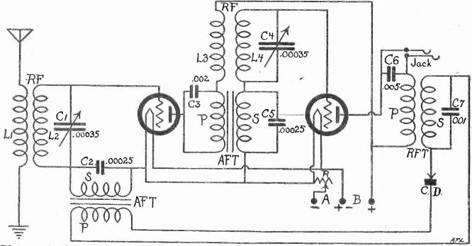
FIG. 144, a 2-tube reflex, employing an Acme radio-frequency transformer, and two General Radio or any other standard make audio frequency transformers. L1 and L2 are both around on a 3" tubing. Use No. 22 DCC., L1, 10 turns, L2, 60. One-half inch separation between the two windings. L3 has 15 turns, L4 has 60 turns, \(\frac{1}{2}\)" between two. Use No. 22 DCC. C. is a fixed crystal detector. 67\(\frac{1}{2}\) volts are employed on plates of tubes. PS is a fixed RFT.
