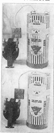
HERE we have the wrong and correct manner in which to correct a by-pass condenser. The top photo shows the lead of the plate post of an audio-frequency transformer going through a by-pass condenser to the positive post, which is wrong. Connect to A— (bottom photo).
