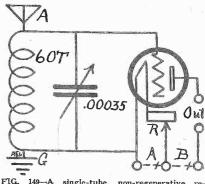
FIG. 149—A single-tube, non-regenerative receiver. This receiver is exactly the same as a crystal set, except that there is more stability and bit more volume. This is the least amount of materials that can be employed in a tube set.
