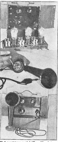
FIG. 7, a resistance coupled AF amplifier that may be connected to the set at home for excellent quality speaker operation. This is the Daven unit. Fig. 8 shows an adjustable speaker unit, with horn, the plug being inserted in a jack connected to the last audio tube's output. Fig. 9 shows front view of setup, with speaker in operation from the set's jack, rewired for audio output.
