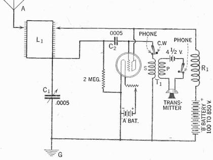
CIRCUIT DIAGRAM of the 5-watt transmitter.
