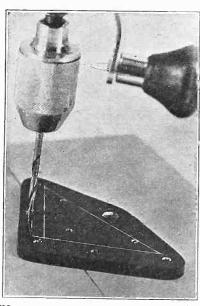
FIG. 3, two holes are drilled outside the triangle, so that mounting screws may be inserted, to enable panel mounting. Since the triangle is to be cut away, the old mounting holes will disappear.
