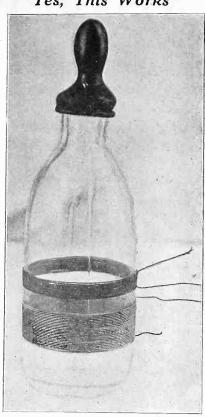
EVEN baby's bottle can be used in a radio set and to advantage. Take some No. 22 or 24 DCC wire and wind 10 turns nearer top of bottle, leave 1/2" and wind 56 turns more. Lo and behold, we now have an efficient radio-frequency transformer of the low-loss type! The coupling can be varied by simply putting the secondary nearer or further away from the primary. This is made easy by the fact that the glass is slippery and offers no resistance as does a bakelite or rubber form.
