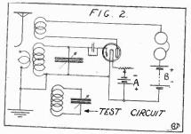
A 3-CIRCUIT single-tube receiver, with a wave-meter placed in inductive relation to the ground. How to construct all types of wavemeters will be described in the Vacation Number, June 6. There is nothing new about this set except that the antenna coil has a switch by which the aerial may be disconnected, so that you calibrate the exact wavelength that your set can receive, without the antenna (which is pure inductance) instead of making the wavelength higher than really the coil will tune to.
