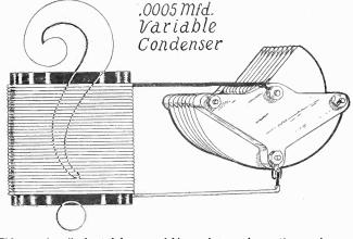
FIG. 146—A coil shunted by a variable condenser. A question mark over the coil shows that a coil which is fixed and can be tuned by a variable condenser, must have an inductance sufficient to be effective with the condenser in shunt to tune the broadcast band. For .0005 mfd. condenser use 43 turns of No. 22 SCC wire for .00035 use 56 turns; diameter of tubing 3½".
