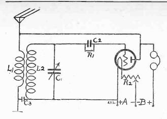
FIG. 147—A diagram of a single circuit single tube regenerative set. L1 and L2 are wound on a 3" tubing. L1 10 turns, L2 60 turns, ½" between two windings. This set oscillates beautifully and is a terrible interference maker. C3 is .001 mfds. C1 is .00035 (usually 17 plates).
