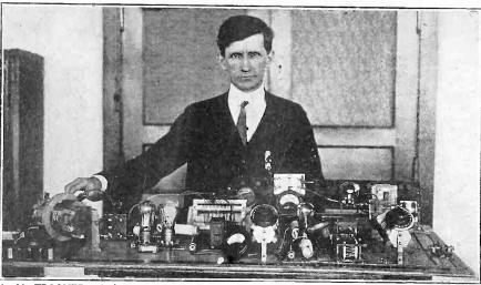
A. M. TROGNER, of the Naval Research Laboratory, operating the short-wave transmitter (40-85 meters) which he designed. This set is to be installed in about thirteen of the Naval Districts throughout the United States. (Harris & Ewing).
