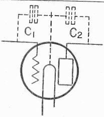
A DIAGRAM shownig in symbols how capacity exists between the grid and plate elements of a vacuum tube. This is the capacity that has to be neutralized in a Neutrodyne receiver.
