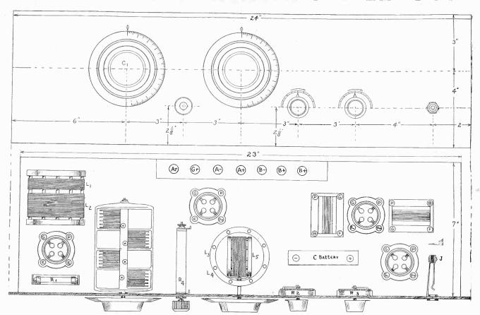
FIG. 2 (top) shows the panel layout. The switches are omitted, as their placement may be at any suitable point. The grid leak knob is between the dials. In Fig. 3, assembly plan, note that the coils are at right angles. This helps present feedback by stray magnetic coupling. R1 is the ballast resistance.
