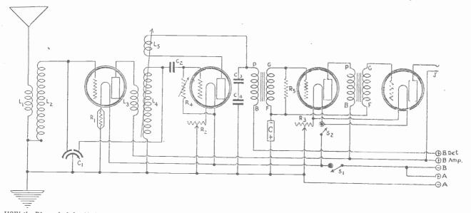
HOW the Diamond of the Air is wired as a 2-control set (Fig. 1). Two variable condensers with a common rotor but with separate stators are used to tune the secondaries L2 and L4. This condenser unit is known as the double or multiple type. The detector grid return is to negative, for it must be the same as the grid return of the RF tube, due to connection to the common rotor. But the variable grid leak goes to A+, and any oscillatory tube may thus be used as detector.
