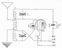
FIG. 1, circuit of the tuned plate regenerative set. The coil terminals are designated by letters, so that the novice will be sure to get the polaritles right. The grid coil CD is connected in reverse fashion to the usual (incorrect) method.
