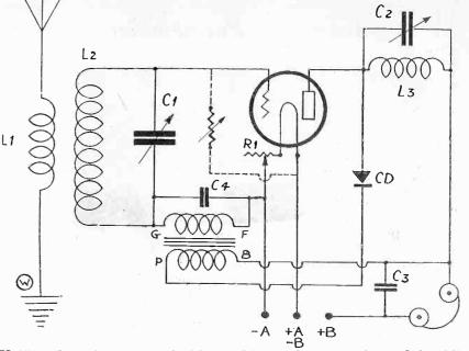
FIG. 143, a reflex receiver using one tube and a crystal detector (CD). R, is a rheestat, Cl is a .005 variable condenser. C2 is also a .005 variable condenser. Li has 10 turns,  $N_{a}^{\prime\prime\prime}$  space is left and then 42 turns put on, No. 22 DCC wire being employed. L3 has 34 turns of number 22 DCC. C4 has a capacity of .002 mfd. The audio-frequency transformer is of the high ratio type.
