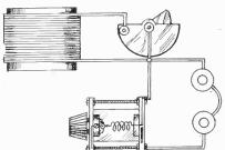
Wavemeter attached. A WAVEMETER hooked up uni-laterally. The components are a 19-turn coil, a crystal detector, a variable condenser and a pair of phones. This instrument is used for calibrating a transmitting station.
