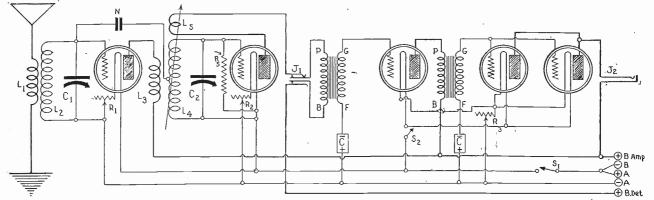
Fig. 1--Wiring diagram of a set having the last audio stage handled by parallel-connected tubes
