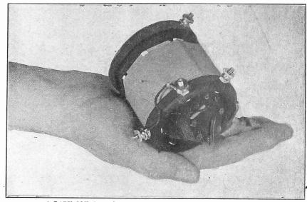
A BABY COIL is used in the 1-B Model Portable for space conservation.
