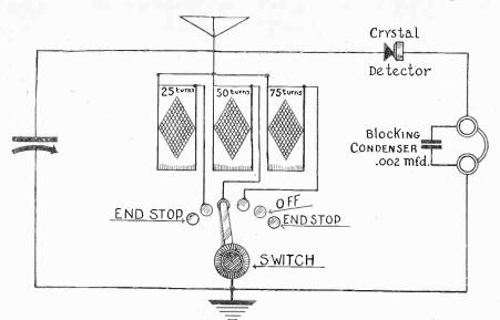
ANOTHER inductively coupled crystal receiver, using three honeycomb colls. This set is more selective than the others shown, on account of the taps on the colls and also the varying of coupling between the honeycomb colls. The condenser which is shunted across the antenna and ground has a capacity of .0005 mid. A long antenna (about 108 feet) should be used. The ground should be run to the cold water pipe. A 3968-ohm pair of phones is used.
