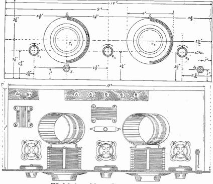
FIG. 2 (top), panel layout; Fig. 3, Assembly plan.
