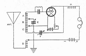
FIG. 1, the wiring of the Reinartz short-wave receiver to be used on Mac-Millan's ship in the Arctic.
