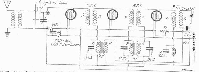
FIG. 142, a 3-tube reflex. A special connection is made for the antenna so that the loop may be inserted without disconnecting or any rewiring of the set whatsoever. The antenna coll consists of 16 turns, the secondary consists of 50 turns, both windings on the same tubing, 3" in diameter, 1/2" separation being left between the windings. Number 22 DCC is used. UV201As are employed. This set is not very selective and is difficult to get working right. The three RFT are of the fixed type.
