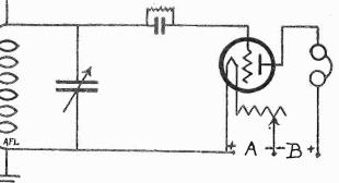
A SINGLE tube, single circuit, non-regenerative receiver. The signals re-ceived in this set are much louder than those from a crystal set, but selectivity is nearly nil. The variable condenser is used for the purpose of tuning the detector circuit in resonance with the antenna circuit.
