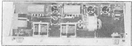
FIG. 4, top view of the Twinplex circuit. The RFT is at left, the coil at right being a 3-circuit coupler, in this instance an Ambassador. The AFT is General Radio No. 285 and the push-pull audio-transformers are those of the Como Apparatus Co. The variable condensers are .0005 Bremer-Tully.
