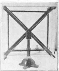
FIG. 5—A view of the completed loop. The type is referred to as box loop, It measures 12" square. A 5%" hole has been drilled in the center-piece so that the stand fits in and allows the loop to be turned freely
