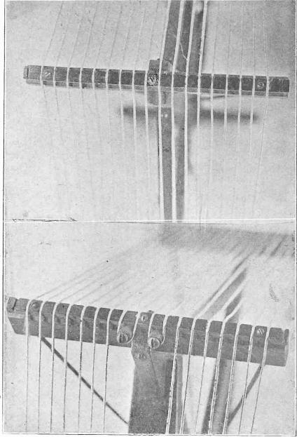
FIG. 8—After you have constructed the box frame of thin pieces of wood, cut four pieces of Bakelite 5" long by ½" square. Then file little notches ½" apart (20 in all) in these Bakelite strips, clearly shown almost full size. These are attached to the four corners of the box frame by
