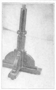
FIG. 1—Close-up of the stand. This measures about 6" high and has been turned from a piece of wood 1" diameter. The little feet, four of which are used, extend out from the sides of the main upright about 2½". Notice the top of the stick which has been turned down to about ½" diameter. This fits into the base of the loop. This is an elaborate device and the same practical effect can be attained by using a ½" dowel stick and an ordinary loop base.
