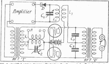
FIG. 2, simplified wiring diagram, illustrating the theory of the Twinplex circuit.
