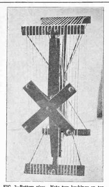
FIG. 7—Bottom view. Note two bushings on top and one on bottom where direction of the winding is changed
