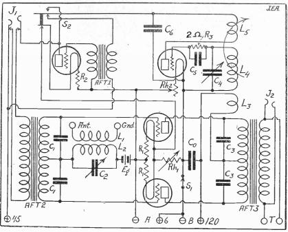
FIG. 1, schematic wiring diagram of J. E. Anderson's Twinplex, where push-pull AF is used for fine quality with great volume. The RF stage is in parallel, being reflexed in the push-pull stages, Mr. Anderson's original idea.
