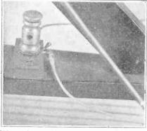
FIG. 2, close-up of the binding posts. Two are used, one for each end of the loop. They are mounted on the base of the loop.
