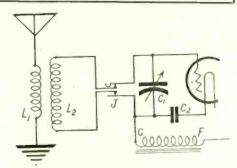
FIG. 102-How to connect a jack for use of either loop or aerial and ground in a reflex set. L1 and L2 are the primary and secondary, re-spectively, of your present set. J is the double-circuit Jack. Connect one outer prong of the jack to the grid of the RF tube, other outer prong to the grid return lead. One of the inner prongs goes to one side of the coil L2 (secondary), the other inner prong to the remaining end of coil L2.
