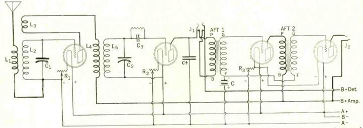
FIG. 1, schematic wiring diagram of the Great 4-Tube DX Circuit, compris ing a stage of tuned radio-frequency amplification, regeneration, detector and two stages of transformer-coupled audio-frequency amplification. This set n ot only gets DX wonderfully but gives great volume and is wonderful in tonal quality.
