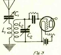
TUNED primary and secondary (left) and impedance coupling.
