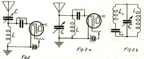
A SERIES condenser tuning the aerial, a parallel-connected condenser in the aerial circuit and the antenna capacity effect (left to right).
