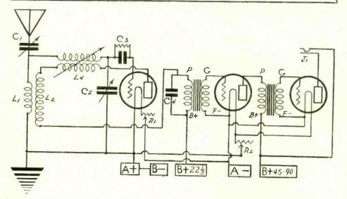
FIG. 100-A 3-tube regenerative set of excellent selectivity and very sensitive. On one spiderweb form having a core diameter of approximately 1" first wind the primary L1 of 40 turns with No. 22 DCC wire. Then wind the secondary L2 with the same gauge wire 60 turns. L4 is the split variometer, the rotor being in the plate lead. CI is 23 plates; C2, 23 plates; C3, a .00025 mfd. grid condenser; C4, a .002 mfd. phone condenser.
