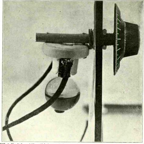
FIG. 9, Hayden's variable grid leak as it looks in completed form when mounted on the panel, with dial affixed.
