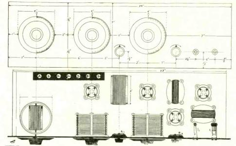
FIGS. 2 AND 3, the panel layout and assembly plan of the Great 4-Tube DX Circuit that uses three-controls. The C battery may be placed at any convenient spot.
