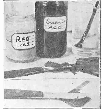
FOR the positive plates a paste is prepared of the ingredients shown in Fig. 7, top photo, and a knife is used (Fig. 8, lower) to press the paste into the drilled holes.
