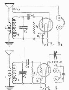
FIG. 1, top, the inductive tickler regenerative set, known as the 3-circuit tuner, employing aperiodic primary. This hookup works well on short-wave work, as does the other, Fig. 2, which embodies a fixed coil in the plate circuit. This plate coil, L3, is tuned by a variable condenser to obtain regeneration through the internal capacity of the tube.
