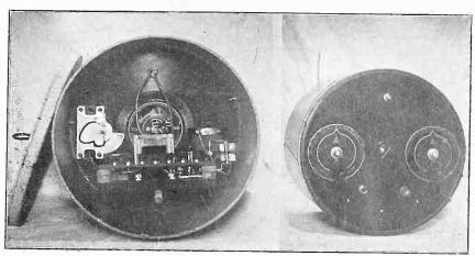
USING a phonograph record as a panel for a portable radio set the result is shown above. The material in the record is a very good insulator. Note the space inside for batteries. (Kadel & Herbert)
