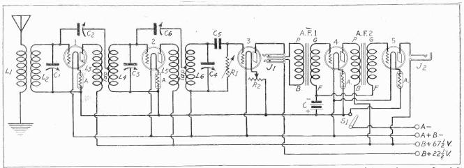
FIG. 1, the circuit wiring of the Low-Loss Neutrodyne. The coils L1L2, L3L4 and L5L6 are basket-weave. The neutralizing condensers are C2 and C6. A C battery is used to bias the audio tube grids. S1 is a master switch, push-pull or toggle. One rheostat is used (R2 in the detector circuit). A represents ballast resistances. They, like the rheostat, should be in the negative A battery lead, as shown.
