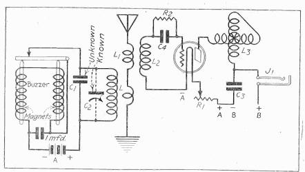
FIG. 1, showing how the unknown capacity of a condenser (fixed or variable) is determined by the wavemeter test. L1 is the regular aperiodic primary of a receiver and L a small extra winding (6 or 8 turns) in inductive relationship to the wavemeter coil next to it. No variable condenser is needed on the receiver.
