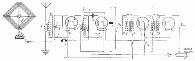
FIG. 1—The wiring diagram of The Diamond of the Air as a 2-control set, with option of loop or aerial operation. L0 and L2 must be matched and the loop must be matched with them, too. Various methods of accomplishing such matching are discussed in the text.
