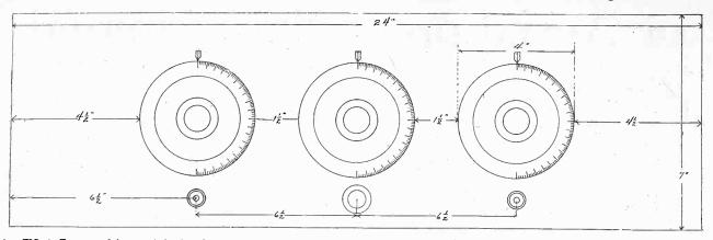
FIG. 3.-Front panel layout of the Low-Loss Neutrodyne. The switch may be inserted in the left-hand corner or right-hand corner of the panel
