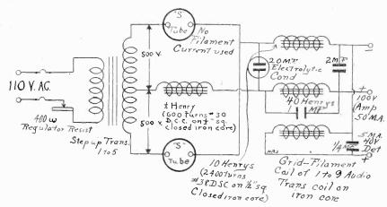
FIG. 2-How to use S tubes in the rectifier unit.
