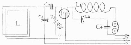
FIG. 3—A 1-tube loop set that brings in local stations. The range is about 50 miles, often much more. It is a good circuit to use to calibrate C1 as against inductance L, which is the loop. C2 is .0005 mfd., L1 is 45 turns of No. 20 DCC wire on a 3½-inch diameter. C4 is .002.
