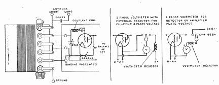
FIG. 20—The diagram at extreme left shows how to wire up the first detector in the Silver Super-Heterodyne, so as to use an antenna and ground. See text for description of coil. The sketch second from left shows how to connect up a filament and plate voltmeter and the next one how to connect up a plate voltmeter only. The voltmeter resistor is wound on a 3" tubing with 500 turns of No. 36 enameled wire.
