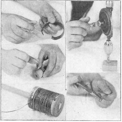
FIG. 1, top left, removing resistance wire from an old rheostat. Fig. 2, on an ordinary spool wind this wire. The completed winding is shown in Fig. 3, bottom left. Cut a block of wood I" thick and 2" square (Fig. 4, top right). Drill a ¼" hole, to insert a dowel stick, take an old switch arm, bend it back a little. See Fig. 5. (Hayden).
