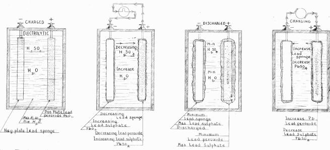
Fig. 1—The picture tells the saory. In the last diagram "Pb" should read "Pb02." In the extreme left-hand diagram the solution called electrolytic should
