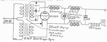
FIG 3-Using a 6-volt bell-ringing transformer and a UV201A to step-up and rectify AC for use on plate of amplifier tubes.
