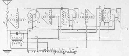
FIG. 1—The circuit of the 3-tube reflex. Three tubes operate as four, the RF being reflexed with the first AF. Distance comes in beautifully and tone is absolutely under the control of the operator.
