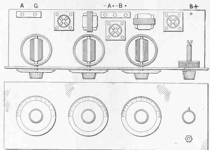
FIG. 2 (top)—The panel layout. Three variometers are mounted on the panel. These three instruments will take up approximately 15". The sockets and AF transformers are mounted in back of the variometers, the rheostat and lack to the right of the panel. Fig. 3 shows the baseboard layout. Three variometers, three sockets, two AF transformers, rheostat and lack are mounted on the 7 x 17" baseboard and 7 x 18" panel.
