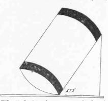
FIG. 79—Getting the correct angle for the Neutroformers in the Neutrodyne. The angle is 57.3 degrees, and to get the proper neutralization of the RF circuit the coll must be mounted at this angle. Place the coll against the angle as shown, after cutting the angle out of the sheet. The side of the angle must be parallel to the odge of the panel, assuming the panel corners are exactly 90 degrees
