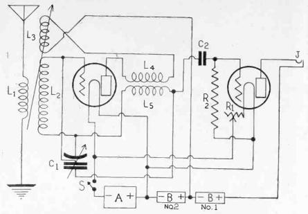
FIG. 14, the 1925 model Superdyne, without the audio stages. This affords only earphone service. To operate a loudspeaker, often on stations thousands of miles away, the two audio stages are vital. The tone quality of this circuit is unsurpassed by that of any other tube set.
