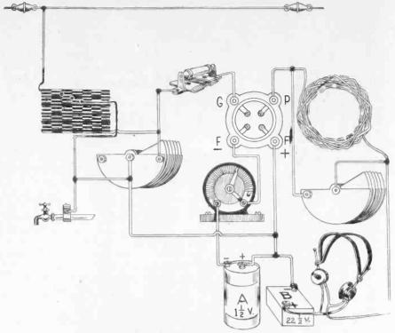
FIG. 4, wiring diagram of Lieut. O'Rourke's set shown in picture form. This diagram simply presents in another form the same wiring shown schematically in Fig. I.
