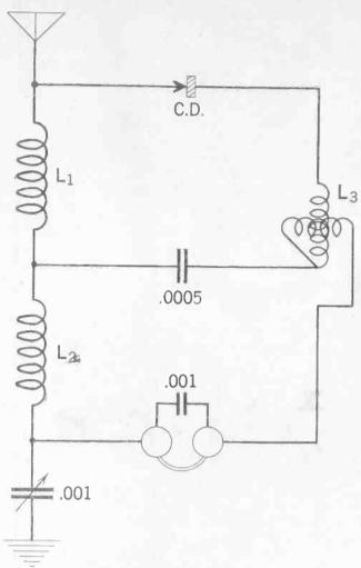
A FAIRLY SELECTIVE crystal set (Fig. 1), constituting an improvement on most crystal hookups. A variocoupler L1 L2 and a variometer L3 are the only inductances used. The third tuning control is the variable condenser C1, .001 mfd, 43 plates. C2 and C3 are fixed condensers. This set may be made for \$15, including earphones.
