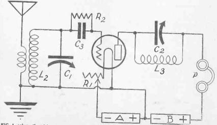
FIG. 1, schematic wiring diagram of Lieut. Peter V. O'Rourke's 1-tube DX set which may be logged and on which the tuning may even be done in step, with any given station coming in at the same dial readings for each of the two controls. Low-loss coils and condensers are used. The condensers are used. The condensers designation fell off the aerial-ground coil. L1, L2 are really one coil, tapped. The coils are home-made.
