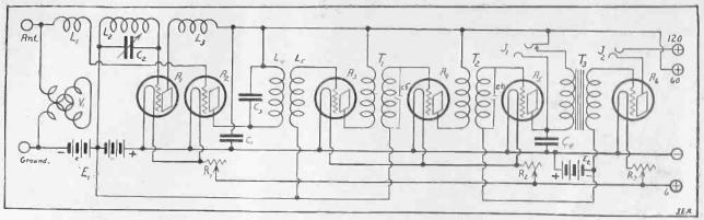
FIG. 88.—The 6-tube Super-Heterodyne. This set will operate very efficiently on a loop, DX results are good, tone good and selectivity excellent.
