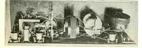
FIG. 7, rear view of the interior. The coupler is at right, the variable condenser next to it, then the radio-frequency transformer, which is tuned by the same variable condenser that tunes the coupler secondary. (RADIO WORLD staff photo.)
