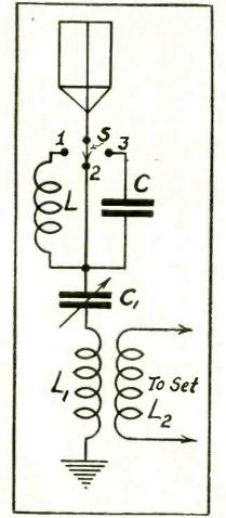
FIG. 2, showing the aerial and ground at top. and bottom respectively. L, L1 and L2 are colls, represented by series of loops. A condenser is shown by two parallel lines (C), while, if variable, an arrow intersects the symbol. This diagram shews how to use a loading coll L and fixed series condenser C for varying the aerial's wavelength electrically.
