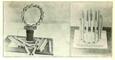
FIG. 6—An anticipatory glimpse, showing what the completed coil will look like, and revealing the spool of primary wire, dowels and block with template pasted on it. Note that on this particular coil an aperiodic primary has been wound of dark-covered wire, to distinguish it from the whitecovered secondary.
