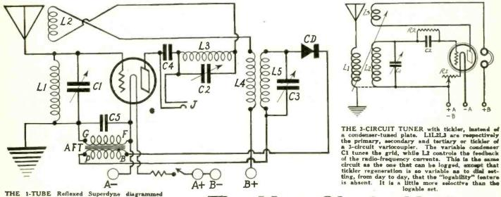
THE 1-TUBE Reflexed Superdyne diagrammed above, affords fine signal quality because of the erystal used as the rectifier. This circuit is not selective enough for those living in cities. L1L2 are both on one tubing and are fixed coupled. All the coils may be made at home. There are three centrols, the variable condensers C1, C2 and C3. This is a good reflex for the beginner to build. It is not a DX set. The circuit was described in the December 6 issue.
