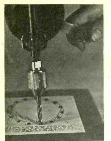
FIG. 5-Showing wrong way to drill.
