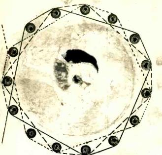
FIG. 2—Template for making the wooden block and inserting dowel rods to wind the low-loss coil. The rods are inserted in drilled holes and are at right angles to the base. The wire is wound in and out of alternate pairs of rods. The solid line represents one turn, the dotted line the next turn and the dash line the next. The coil is made self-supporting. The diameter between dowel centers is 3 inches. strictly technical things like grid biasing and the prevention of stray coupling.
