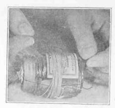
FIG. 5—The two terminal of one of the cut pieces of thread are removed and the thread knotted around the new winding, which wil constitute the primary. This operation is repeated three times.
