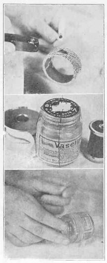
FIG. 2 (top) shows how sealing wax is used to bind the new end of the coil. The middle photograph (Fig. 3) shows how two pieces of thread wound the length of a small vaseline bottle and secured on top with adhesive tape. The roll of tape is at left. At right is the spool of thread. Fig. 4 (bottom) reveals the method of winding the excess wire, taken from the honeycomb coil, right on the vaseline bottle.
