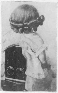
TWO DIALS keep this Baby Doll in tune with the universe. The doll contains a 3-tube set, loudspeaker unit and horn.
