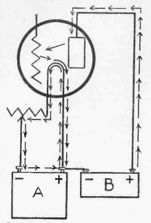
FIG. 2, the path of the direct current in the tube. The current travels from negative to positive. One filament lead (in this case F+) is a common conductor of A and B battery current
