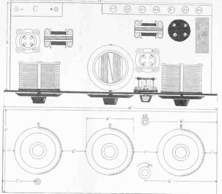
FIG. 3, combined panel layout and assembly plan for the Bluebird Reflex.
