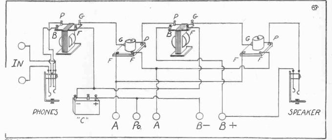
FIG. 77-A 2-stage audio amplifier illustrated. The IN is connected to the plate and plus B detector battery. AC battery should always be used on the amplifier to clear the tone and save the B battery.
