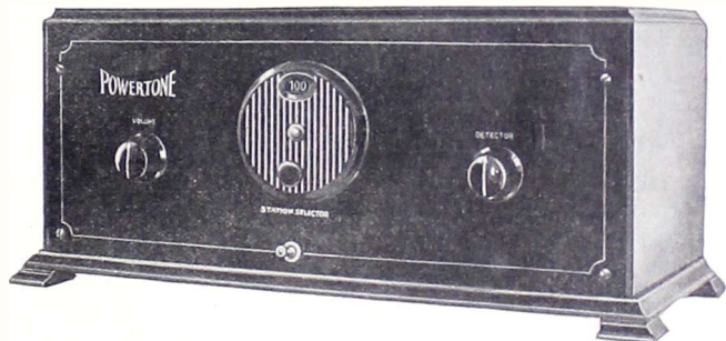
THE PANEL VIEW of the Powertone is a cabinet. The panel is 7x18". The dial is in exact center, while the switch is just underneath it. The rheostats are disposed at equal distances to left and right of the sides. The dial causes the tuning to be on a straight line frequency basis when a double condenser is used that is not SLF.
