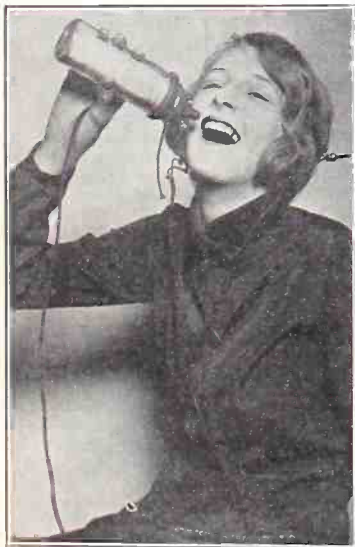
VIRGINIA NORTON listening in on a "Baby Bottle" crystal set. This was one of the interesting amateur exhibits at the Radio Show in Chicago. The coils are wound on the inside of the bottle and crystal and taps on the rubber nipple. (Underwood & Underwood).
