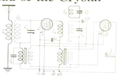
ONE STEP FARTHER and we have a reflex set that works a loud speaker and which is selective. The wave trap idea is retained. This is the same as Fig. 4, except that a second stage of audio (this one not reflexed) is added. (Fig. 5.)
