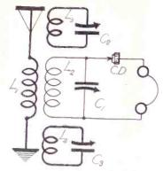
A SELECTIVE CRYSTAL SET for a point of reception that has a 3-station range. Any one of the three stations may be tuned in by Cl, the two others tuned out by the wave traps, L3C2 and L4C3. As the primary L1 is not tuned there is no compensating effect and the set may be logged. (Fig. 1.)
