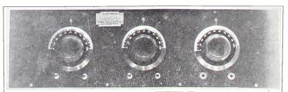
FIG. 4, showing the front panel view of the set...The first dial controls the shaft of the variable condenser shunted across the second RFT and the other dial controls the shaft of the condenser shunted across the secondary of the detector coil. The other dial controls the rotor of the variometer.
