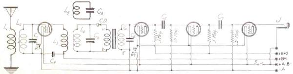
THE SAME CIRCUIT as shown in Fig. 6, except that the first audio stage is not reflexed. (Fig. 7.)
