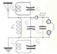
A TUNED IMPEDANCE primary gives more volume than the inductive coupling method shown in Fig. I, but the set suffers in selectivity. Under certain conditions, explained in the text, this hook-up is very good. (Fig. 2.)
