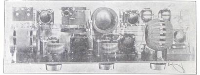
FIG. 3, looking down on the receiver. This photo gives a good idea of how the parts should be placed on the baseboard.
