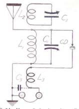
FIG. 3A—How a 3-circuit tuning coil may be employed in a wavetrap crystal hookup. L1 is the rotary coil. L2 is the secondary (large stator winding, used for trap). L3 is the otherwise aperiodic primary. The rotary coil L1 is loosely coupled and left that way.
