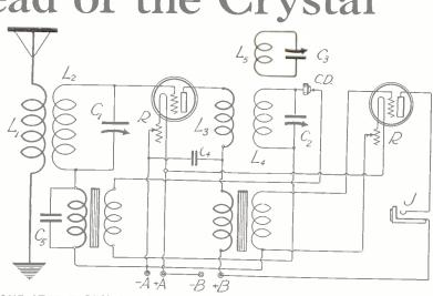
ONE STEP FARTHER and we have a reflex set that works a loud speaker and which is selective. The wave trap idea is retained. This is the same as Fig. 4, except that a second stage of audio (this one not reflexed) is added. (Fig. 5.)
