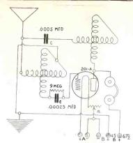
FIG. 189, showing a receiver employing 1-Tube, the grid and plate being tuned by variometers. The rheostat has a resistance of 10 ohms. When building this set, place the variometers no more than  $23_4^{\prime\prime\prime}$  away from each other. The mid-tap is taken
