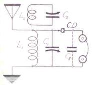
INSTEAD of two wave traps one may be used, but that is efficient only if the receiver has a 2-station range. (Fig. 3.)
