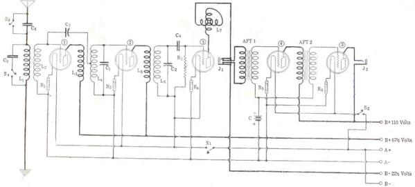
Fig. 1, showing the electrical diagram of the Improved Diamond. "here are 5 tubes in this set instead of 4 tubes as in the original Diamond.
