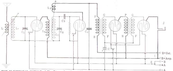
THE ELECTRICAL WIRING of The Diamond, with variable antenna coupling (Fig. 185)., L may be the tickler of a variocoupler, L0 a secondary made to match the condenser Cl. The set will have four controls, unless ClC2 is a double condenser, whereupon there are three controls. L need be varied only occasionally, hence the set would be practically in the 2-control class. Constants are given in the May 23 and July 25 issues of RADIO WORLD.
