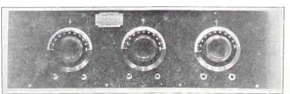
FIG. 4, showing the front panel view of the set... The first dial controls the shaft of the variable condenser shunted across the second RFT and the other dial controls the shaft of the condenser shunted across the secondary of the detector coil. The other
