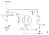
FIG. 1, wiring diagram of the electrostatic regenerator.
