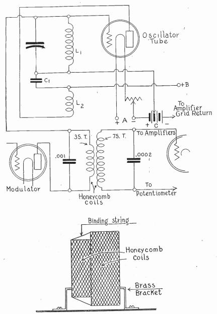
FIG. 128 (top), grid return of Benson's Super-Heterodyne included. Lower, detail of fil oscilator to C minus, with a filter circuit filter construction
