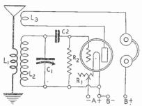
FIG. 1, the standard 3-circuit regenerative set, very selective and suitable for all locations. It works on either an indoor or outdoor aerial. CI is .0005 mfd. C2, the grid condenser, is .00025, while the grid leak should be variable. Once the right leak setting is determined it need not be changed. Note the rheostat is in the negative leg.
