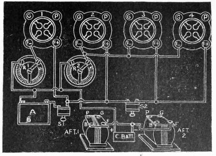
FIG. 6, showing how the filament connections are made in "The Diamond of the Air."
