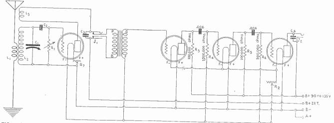
FIG. 1, circuit diagram of a 3-circuit tuner, tickler variety, with three stages of audio-frequency amplification. coupled, the two others resistance-coupled, Daven resistors being used. The first audio stage is transformer-
