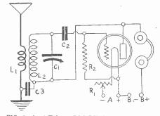
FIG. 5, the 1-Tube, 1-Dial DX Set, where, as in Fig. 4, the rheostat controls regeneration. This circuit was described in the December 6 issue. The fixed condenser C3 connecting primary and secondary is .001 or .002 mfd.
