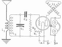
FIG. 3, the same effect as obtained from tuning a fixed coil by a variable condenser may be enjoyed by putting a variometer in the plate circuit. The same principle is involved, a form of capacitative coupling of plate to grid, through the internal capacity of the tube, that is, the condenser effect existing between the grid and plate elements. Tuning the plate accomplishes this internal transfer. C3 is .001 or .002 mfd.
