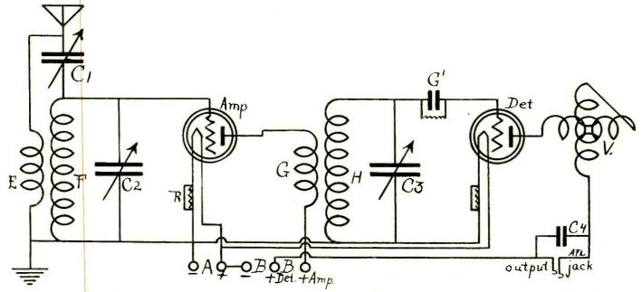
THE OSCILLATIONS in this circuit are kept under control by the condenser C1, which, when at a setting to be determined by experiment, will keep the tube at its most sensitive point. This setting may remain, hence there are three active controls in the circuit, not four. Both coils, EF and GH, are the same, E and G being 5 turns and F and H 50 turns, No. 22 DCC wire. All the variable condensers are 23-plate and must be low-loss for best results.
