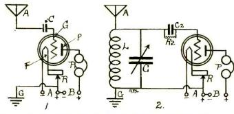
FIG. 1, A, antenna; G, grid; P, plate; F, filament; Ph, phones; R, rheostat; G, bottom, ground. In Fig. 2. L is a coil; C. a variable condenser; C2, grid condenser; R2, grid leak.
