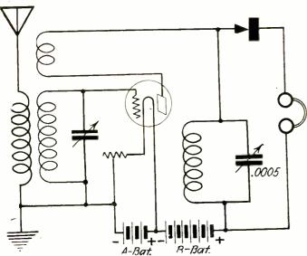
FIG. 34.—Crystal detector used in Superdyne.
