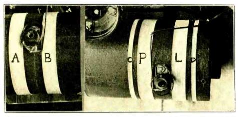
TWO VIEWS of the stator windings are shown in Fig. 7, above, at left. For Figs. 1 to 6, inclusive, see front cover. In Fig. 7 A has 20 turns of No. 26CCC wire, and so has B, but B is tapped at its tenth turn, or the thirtieth turn from the beginning, because A and B are a continuous winding. The tap is carried out to binding post No. 1. (See Fig. 2 on front cover).
