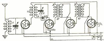
FIG. 3.—The wiring diagram for Caldwell's 4-tube set, consisting of one stage of radio-frequency, detector and two stages of audio-frequency. Radio-frequency transformers are basket-wound, low-loss type. The use of low-loss condensers increases the efficiency to make this set almost the equal of a 5-tube receiver.
