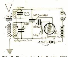
FIG. 35.—Diagram of a 3-circuit tuner using honeycomb coils.
