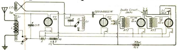
THE FAMOUS SUPERDYNE circuit which has held the interest of thousands of fans since its inception. Coils L, L1 and LF1 compose the variocoupler, and coil L2 is the plate coil. The use of the grid leak as shown is optional, as in many cases better results are had by placing from the grid post to the positive filament post on the socket. With low loss parts this circuit is said to be the equal of a 6-tube set, and is noted for its extreme clarity.
