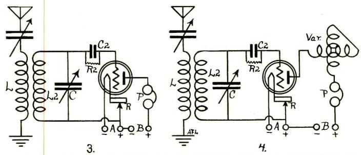
FIG. 3, simple vacuum tube detector circuit using variocoupler. R2, the leak, is optional with some types of tubes. Fig. 4 shows the addition of a variometer in the plate circuit which causes regeneration. The rest of the circuit remains the same as in Fig. 3.
