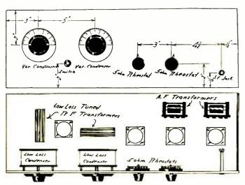
FIG. 1 (top) shows panel layout. The panel should be some high-grade insulating material 7"x21" on which are mounted the two condensers, rheostats, jack and filament switch. Fig. 2 shows the instrument layout. The RF transformers should be mounted at right angles and the audio-frequency transformers kept as far away as possible to prevent audio-frequency feed back into the radio-frequency tubes, which causes howling. This layout will give the short leads necessary for efficiency.
