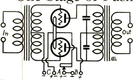
FIG. 38.—Push-pull power amplifier circuit asked for by Frank Baertich of Troy, Indiana. The transformers are purchased in pairs and are matched. Ninety volts are used on the plate and one rheostat controls both tube filaments.
