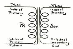
HOW the connections are made to an audio-frequency transformer. The plate lead, if this was the first AF, would be from the detector tube.
