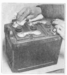
FIG. 6—The storage battery must be kept frea from corrosion. A batery whose terminals are covered with corrosion, is a battery whose life will be comparatively short. Keep the battery clean and you will be rewarded with long, care-free service.
