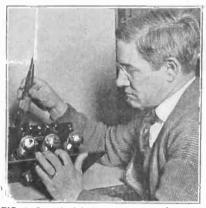
FIG. 1—Dust is injurious to any set, but especially in a Neutrodyne. The neutralization must be exact and is very critical. Dust increases the capacity of the transformer and is likely to throw the entire circuit out of neutralization. Neutrodynes when out of neutralization are uncontrolable in their oscillation. Keep the set in a tight cabinet, and dust thoroughly at least every six months.
