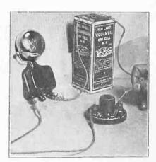
This shows how the lightning arrester is FIG. 5—This shows how the lightning arrester is placed for a short-circuit test. Almost all instruments may be tested with just this apparatus—a battery and a bell or buzzer. The coil may be tested for continuity by substituting the coil for the arrester. If the bell rings coil is all right. Variable condensers and lightning arresters placed in circuit should not cause the bell to ring. A ringing bell with condenser in circuit indicates a short.
