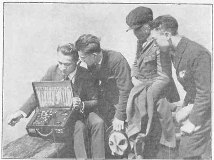
(Kadel & Herbert) HERE is Sidney Kasendorf again, this time with a summer product, a two-tube portable reflex, with even the batteries enclosed in the neat case. Sidney, otherwise 2ATV, uses a fishing line for aerial and ground. This line is wound on a regular fishing reel, and he says it is about the easiest coil winding he ever attempted.
