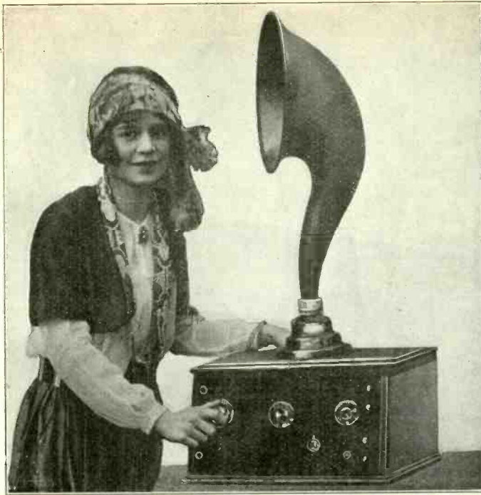
AT the Park Avenue fair, New York City, charming Marie Anferman directed the radio department. The panel view in the picture shows where dials and rheostat should be placed in the Ultra Reflex. Left to right, the dials are variometer, condenser and variocoupler. Two AF stages should be added for loud speaker operation.
