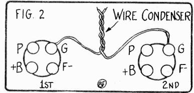
Fig. 2. A simple form of feed-back condenser made of two wires twisted together as the feed-back capacity shown in Fig. 1.
