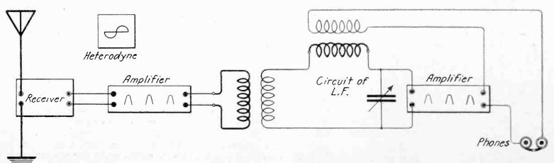
Fig. 1. How the original Lvovitch receiver was worked out. A separate heterdyne was used on the high frequency amplifiers when reception on continuous waves was desired.
