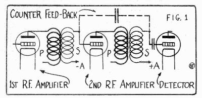
Fig. 1. Self-oscillation in a radio-frequency amplifier may be controlled by using a small condenser so arranged that it feeds back energy of opposing voltage to that which is causing the oscillation.
