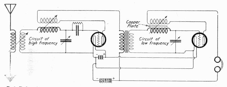
Fig. 2. The Lvovitch circuit as finally developed. It uses but two tubes, with feedback or reactance in both circuits, and a variable copper plate in the field of the second or audio-frequency side.
