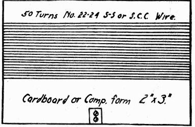
Fig. 3. Tuning inductance used in the receiver. This is the only coil used.
