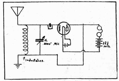
Fig. 4. The circuit is the DeForest ultra audion, single circuit receiver.
