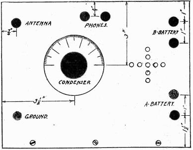
Fig. 1. Panel layout for the single control receiver.
