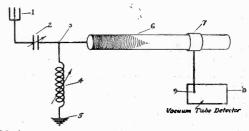
Method of using a tuned resonance coil for the reduction of interference as well as electrostatic disturbances.
