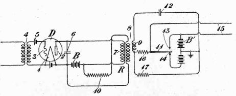
Means for including a sensitive relay in the plate circuit of a receiver.
