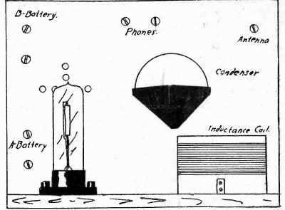
Fig. 2. The interior of the set, showing location of the apparatus.
