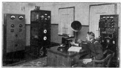
Operating room of Station WCBD, Zion, Ill. On the extreme right is the Western Electric speech amplifying control board. In front of the operator on the opposite side of the room are the transmitter control panel and the transmitter tuning panel.
