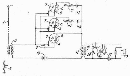
Means for reducing static disturbances by stabilizing them against the received signal energy
