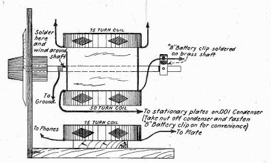
Schenck's method of reaching all the broadcasting wave lengths very conveniently on the Gordon receiver by the simple use of two different sized antenna coils on a movable axis.
