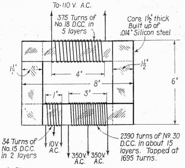
Fig. 1. Diagram showing location and winding of coils on the transformer.
