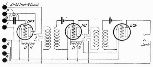
Detector and two stages of audio-frequency amplification with "C" batteries asked for by Kenneth H. Jones.
