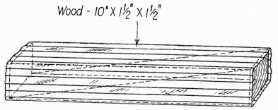
Fig. 2. Wood former used to wind the coils of the transformer. It is easier to wind it on the wood block than on the laminated leg.
