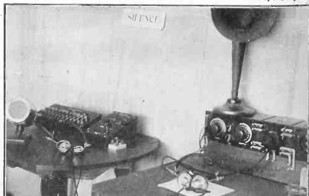
ANNOUNCER'S microphone and control station in the Hotel Mt. Royal, Montreal, where programs are picked up and carried to station CKAC, La Presse, Montreal. The control panel which switches the different halls to La Presse station is at the left, and on the right is the receiving set which guides the operator as to volume and quality
