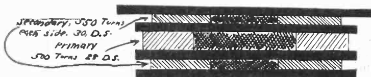
FIG. 2 (left) shows the end forms for the intermediate frequency transformer windings, made square for the radio fan's convenience in constructing. The cutting dimensions are given on the diagram. Fig. 3 (above) is a cross-section view of the completed intermediate-frequency transformer. The primary is wound on one form and the secondary wound in two sections—one placed on each side of the primary. It is of the utmost importance that both sections of the secondary winding go in the same direction, otherwise the set will not work. The primary has 500 turns No. 28 double silk covered wire, and each section of the secondary 550 turns of No. 30 double silk covered wire. Fig. 4 (below) is the panel layout correctly measured and marked off so that the builder can follow the dimensions and be sure that all the holes will be in their proper places. The best way is lay out on a piece of wrapping paper the exact size of the panel and all the holes to be drilled. Paste this on the actual panel and drill through the marked places. The paper is easily removed by soaking the panel in warm water.
