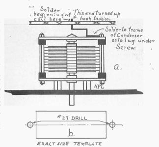
places. This will form one solid piece of wire of double strength for the support. Bend the wire as shown in Fig. 2A and cut it, figuring on hanging the coil about ½" back of the condenser as shown. This support will easily hold up the plate coil rigidly and it disposes entirely of the necessity of any other means of support employing insulating material and metal screws.
