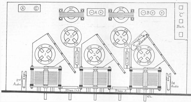
FIG 5, assembly layout, top view, of Magnadyne. The neutralizing condensers are not shown in this diagram as they are supposed to be hidden underneath the variable condensers and anyway their position is optional. No binding posts are provided for the C battery, as the battery is already provided with clips.
