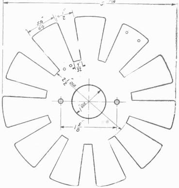
FIG. 1—Schematic layout of the antenna tuning inductance, giving cutting dimensions. Starting at the inside, wind three turns of No. 24 DSC wire and make a small loop for a tap. Continuing, wind seven more turns in the same direction and make another loop for the second tap. Without breaking the wire, wind 43 more turns of wire and terminate. The total will be 55 turns of wire, or about sixty feet. The spider-web form is 5 inches in diameter and ½ inch thick. See page 6 for actual size template.
