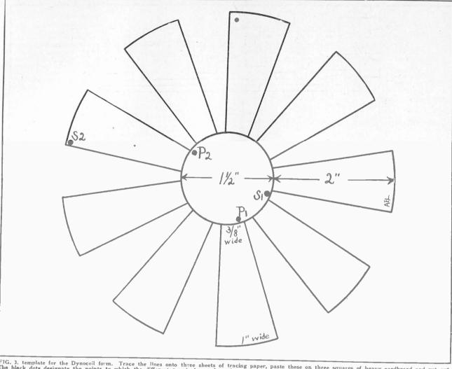
FIG. 3, template for the Dynocoil form. Trace the lines onto three sheets of tracing paper, paste these on three squares of heavy cardboard and cut out. The black dots designate the points to which the different terminals are brought. After the windings are completed, the coils are bound with thread and the form extracted thereby, forming a low-loss coil. The template is exact size.
