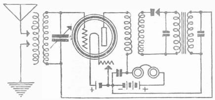
FIG. 5. Reflex circuit diagram asked for by J. O. Applegate
