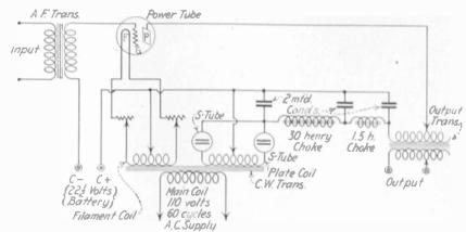
ONE TUBE power amplification, using filament transformer.
