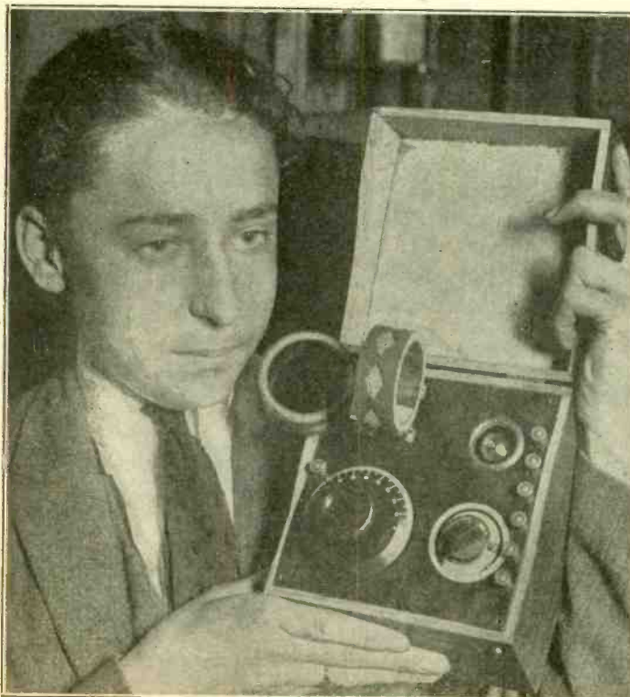
(C. Kadel and Herbert) A miniature receiver made by Alexander Udoff, 16-year-old New York amateur builder. It is the Flewelling receiver, uses one UV199 tube and is a most complete and compact device. Take note of the very careful wiring and the manner in which the tube socket has been mounted to conserve space.
