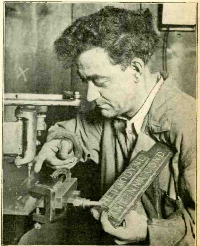
(C. Kadel and Herbert) The main reason that an amateur can never make a good job of engraving panels. Contrary to general opinion the work is not done by hand, but by means of this engraving machine. The brass matrix shown is placed on a machine resembling a pantograph, and the revolving drill point does the actual work, without troubling about the small details.
