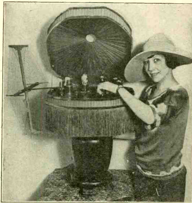
(C. Kadel and Herbert) One of the most interesting commercial exhibits at the exposition was this radio lamp. It is a combined table lamp and radio receiver, with the loud speaker in the base of the lamp. It is made in either the three, four or five tube combination, operates on either antenna and ground or small loop, and has but one tuning control no matter what system is used.
