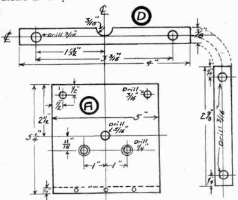
Fig. 2. Panel layout (A) with correct drilling dimensions for all holes. Brass brace (D) to enable the coil to be mounted on the panel without drilling additional holes.
