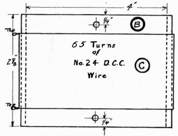
Fig. 3. Dimensions of cardboard or fibre tubing (B). Winding for wave trap (C). This tubing is drilled as shown, according to the dimensions marked.
