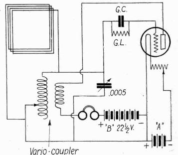
Fig. 2. Another adaptation of the same circuit. Slightly more complicated in control, and less selective, but more range and volume on local stations. Tickler feedback regeneration is used.
