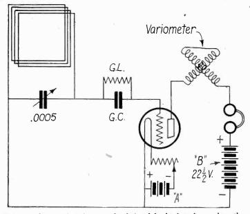
Fig. 1. A loop receiver for one tube designed for local work, or where the listener does not desire to operate a loud speaker. Good for 25 or 30 miles under ordinary conditions.
