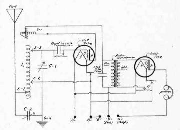
Two-tube receiver which is extremely selective and very flexible as to control and tuning.
