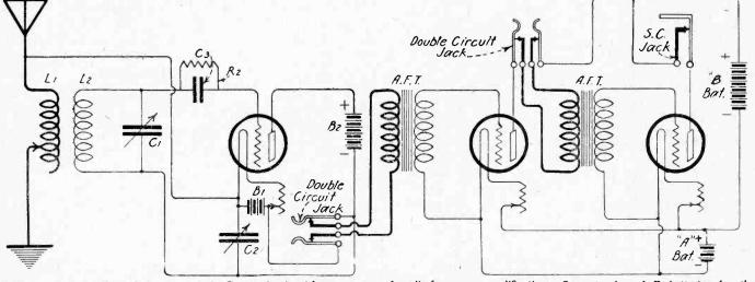
Circuit asked for by E. R. Siebert. It is the Potter circuit with two stages of audio-frequency amplification. Separate A and B batteries for the amplifier work best with this receiver, due to the peculiar method of coupling used in the Potter receiver. Use the same constants for detector as in the Potter circuit.
