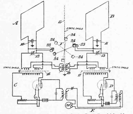
Receiver embodying several new and distinct ideas in radio reception. A balanced loop system is used which, when combined with the apparatus named, provides an extremely sharp-tuning, interference-proof receiver.
