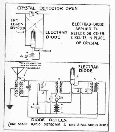
Fig. 1 (below) and Fig. 2 (above) showing the use of the diode tube in a reflex circuit and how it is connected in place of a crystal detector.
