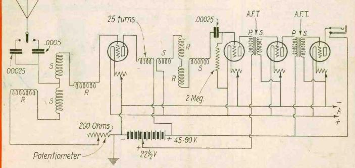
Fig. 1-A four-tube radio-frequency receiver, using split variometers as tuning inductances and radio-frequency couplers. It is possible to operate this receiver on extremely short indoor antennae.
