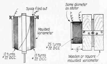
Fig. 2—Two methods of adapting regular variometers for use in this circuit. On the left is the moulded type. The coupling coil is wound on the outside of the moulded composition. On the right the conventional wooden form, adapted to the purpose. The coupling is tight and is fixed.
