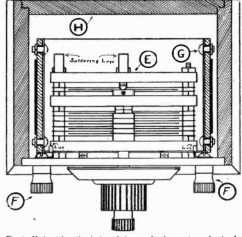
Fig. 4. Horizontal sectional view of the completed wave trap, showing how the coil and condenser are mounted.
