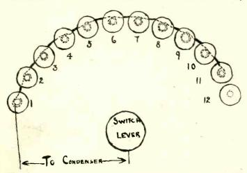
Fig. 1. Method of making a variable grid leak by fastening an India ink soaked string under the nuts of taps.
