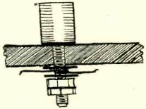
Fig. 2. Method of fastening the string to get good contact. It is wrapped around the shank under the washer.
