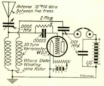
Mr. Turnbull's new circuit which permits the construction of a simple set with but two controls, yet which will satisfy the seekers of super-selectivity.
