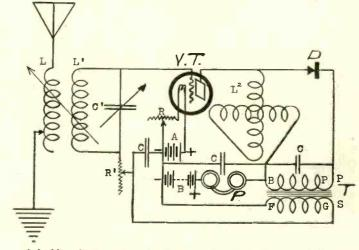
A highly selective reflex circuit using one tube and a crystal detector.
