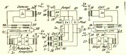
Colpitts' new method of modulating telephone signals.
