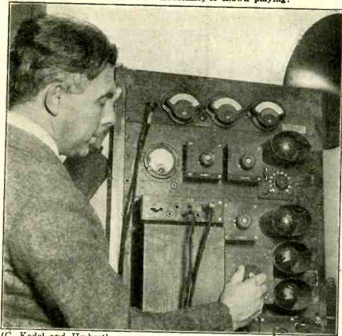
(C. Kadel and Herbert) The speech amplifier control used to modulate the Skinner organ recitals before they are sent over the land wires to the operating room of WEAF. Because of the great volume of sound produced by an organ on the deeper tones it is necessary to regulate the apparatus extremely carefully if perfect reproduction is to be obtained.
