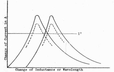
Fig. 5. Resonance curves representing two different waves corresponding to different stations sending at one time.
