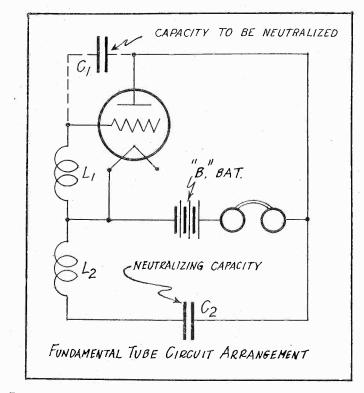
In actual practice inductance coils L1 and L2 may be respectively the primary and secondary inductances of air core radio frequency transformers. The secondaries of these transformers are preferably tuned by variable air condensers. A distinct advantage of the neutrodyne circuit is the fact that radio frequency transformers may be employed having a step-up ratio of windings of the order of one to four.
