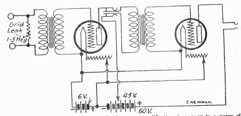
Schematic diagram of two stages of audio frequency amplification, in answer to a query of R. O. Cooke. The grid leak across the primary of the first transformer gives easier control of the high frequency squeal, which otherwise might prove troublesome.
