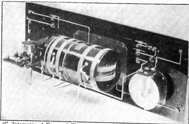
(C. International Newsreel Photo) Illustration of a new receiver which has been perfected by V. M. Moen, St. Paul, Minn., and which is extremely flexible and sensitive. The feature of this circuit is the combined variometer unit shown which is composed of two rotors which take the place of the two variometers and variocoupler in the regular regenerative circuit.
