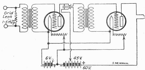
Schematic diagram of two stages of audio frequency amplification, in answer to a query of R. O. Cooke. The grid leak across the primary of the first transformer gives easier control of the high frequency squeal, which otherwise might prove troublesome.
