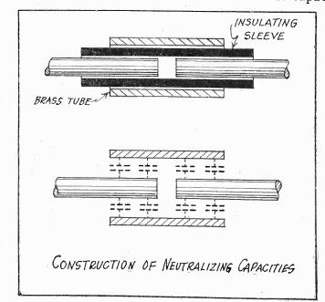
coupling between circuits is reduced to a minimum, if not to zero. The neutralizing capacity may have a capacitance of from 1 to 5 or 6 micro-micro-farads. (Continued on following page)
