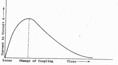
Fig. 4. Showing how, if the coupling is loosened beyond a certain point, the response of the signal suddenly decreases.
