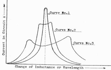
Fig. 3. Three curves plotted for three different values of coupling, showing the difference in the peak of the wave when close, medium, or loose coupling is used.
