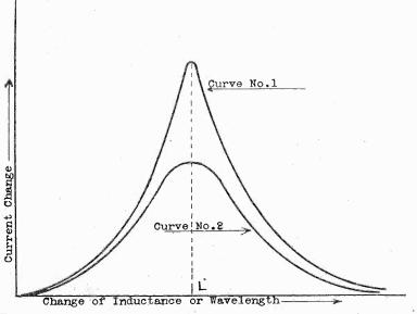
Fig. 2. Curve plotted to show current change as inductance is changed in the circuit.
