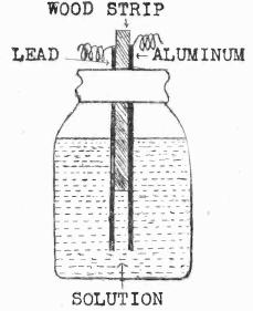
Fig. 1. Schematic drawing illustrating the method pursued in making up and arranging the elements of the rectifier.
