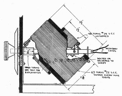
Fig. 1. Constructional details of the coupler described in the accompanying text. The secondary, or rotor, is fashioned to fit on a Z-shaped piece of metal allowing  $180^{\circ}$  variation, which is impossible with the present-day type.
