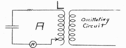
Fig. 1. Illustration depicting tuned primary circuit of a simple set, with ammeter in circuit to show current flow. This is the simplest type of oscillatory circuit.
