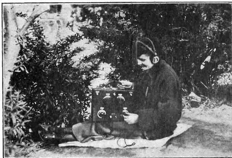
The portable set being used by simply attaching a wire from the center post to the foliage of a convenient bush.
