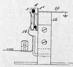
Janson's improved device for protecting electric circuits.
