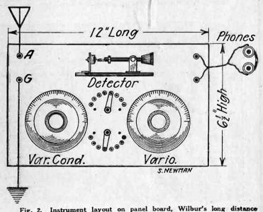
Fig. 2. Instrument layout on panel board, Wilbur's long distance sensitive crystal receiver.
