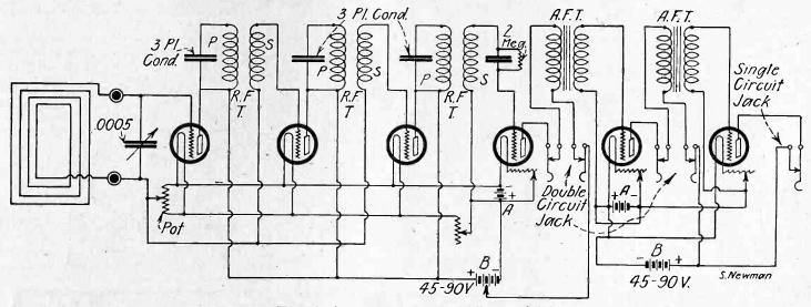
Circuit diagram asked for by C. E. Nordstrom. The radio-frequency amplifiers are all controlled from one rheostat, which simplifies the controls considerably. Separate A and B batteries are furnished for the audio-frequency and radio-frequency tubes to prevent any chance of trouble due to radio-frequency currents leaking through to the audio-frequency tubes. This is the best method of procedure in a set of this type. Tuning is done by means of the condenser shunting the loop.
