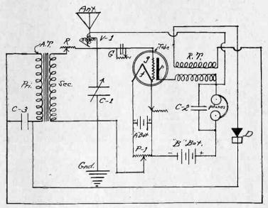
Schematic diagram of a reflex circuit that will surprise and delight the average fan who likes to have a little latitude in the construction of a set. It is important that a good ground connection be used with this set, because of the fact that a single circuit tuner system is used.
