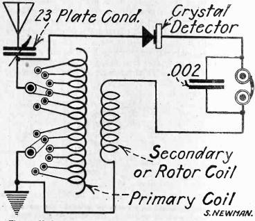
Fig. 1. Hook-up for Wilbur's long distance sensitive crystal receiver.
