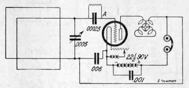
Diagram of a loop set employing the "flivver" principle that will work admirably on a comparatively small loop. Care should be taken in the construction and placing of the condensers.
