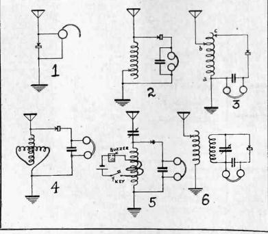
Figs. 1 to 6. Simple circuits suitable for broadcast listeners.
