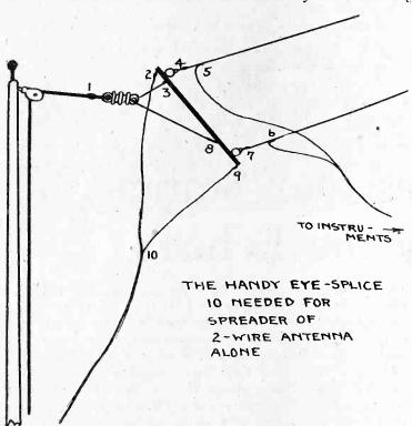
Fig. 1—Showing ten places where the eye-splice can be serviceably used in the erection of a first class antenna.
