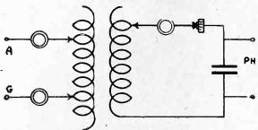
Fig. 1—Circuit diagram to be used with the set described. By connecting a variable condenser across the secondary, greater selectivity and easier control can be had.
