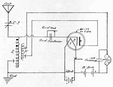
A single circuit regenerative especially adapted to the new U.V.199. Note the fact that the tickler inductance is variable, which adds considerably to the ease in obtaining the critical regenerative point just before the tube "spills."
