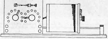
Fig. 3-The complete receiver as it should appear when finished. If care is taken in construction, and a good coat of alcohol stain applied, a very neat and serviceable instrument will be the reward.
