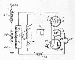
Receiving system utilizing cascade detection and selective feedback.
