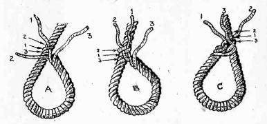
Fig. 2—The three stages of starting an eye-splice in rope. By referring to the text in connection with these sketches it is very easy to splice the toughest rope or the finest line.
