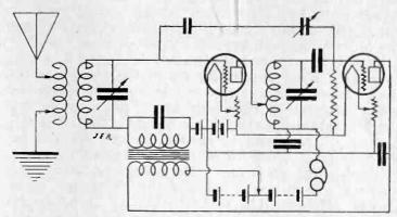
Reflex circuit incorporating the fundamental circuit of the Nite Owl Special. Note the neutralizing capacities which are used to prevent the tube from oscillating.
