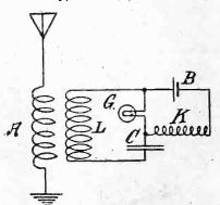
Means of measuring wave length by sight.
