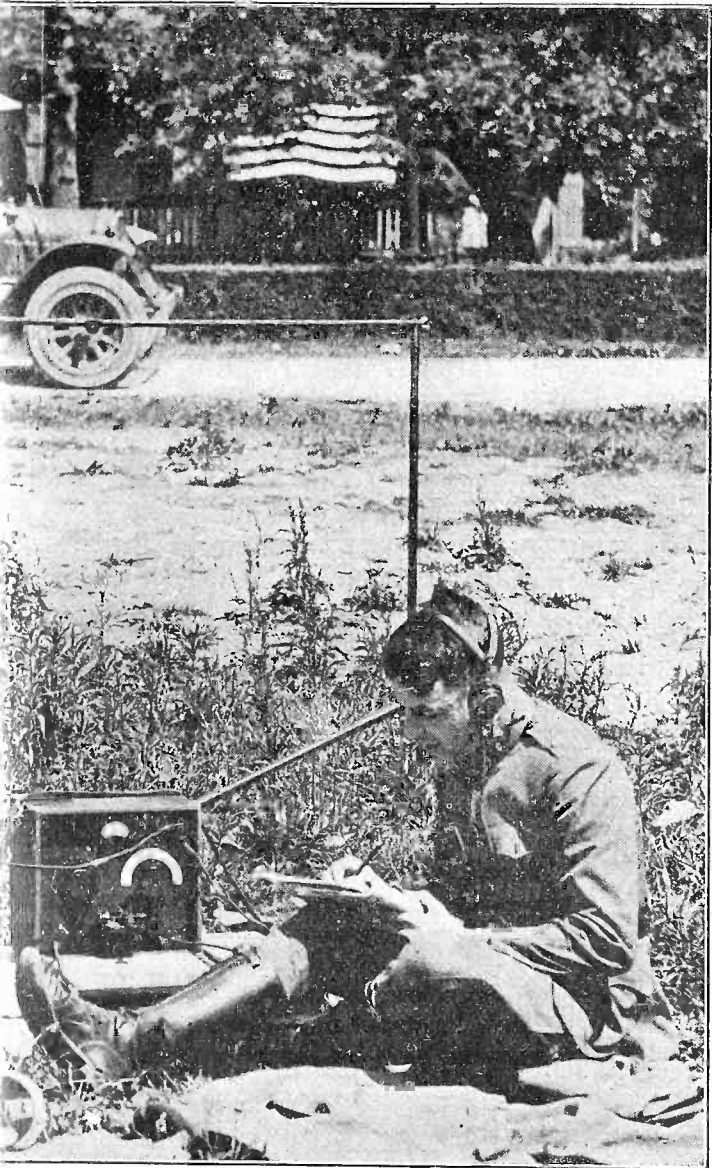
g with short wave receiving and transmitting over small loops. This here are 115 men and officers of the United States Army at Camp their energies are devoted to transmission and reception over the status used for these waves is extremely portable and two men can waves. Note the fact that the loop is portable and can be folded two feet in length.
