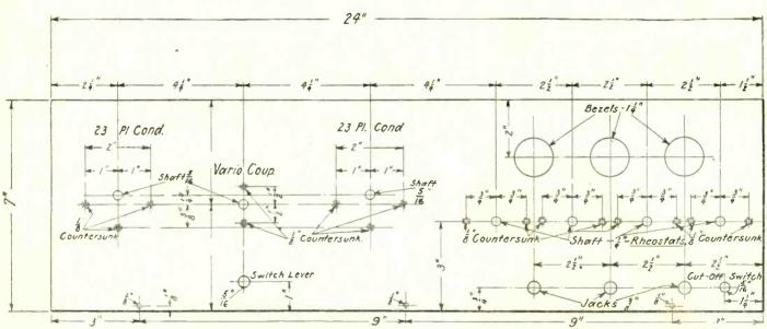
Fig. 1. Panel layout drawn to exact scale. All measurements given are for standard parts unless specific apparatus is mentioned.
