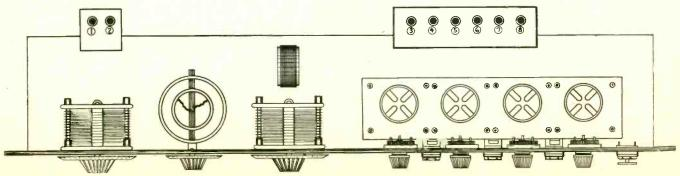
Fig. 3, Top view of the apparatus mounted on base and panel. Binding posts 1 and 2—antenna and ground. 3—A minus. 4—A plus. 5—B minus. 6—B plus 22½. 7—B plus 45 volts for R. F. tube. 8—B plus amplifier (67½ volts).
