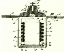
Improved condenser of the sectional type designed for high tension work.
