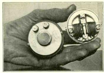
A phone which is popular in England, and has been found to make a good loud talking unit over here—the Brown telephone unit, one of the first phones to make use of adjustable field pieces, showing the "works" as well as the screw which makes the fine adjustments possible. The unit stands quite heavy plate currents without undue distortion and rattling.
