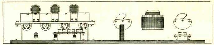
Fig. 2. Rear view of apparatus as mounted. Note mounting of sockets to accommodate transformers. The binding posts project through back of cabinet.
