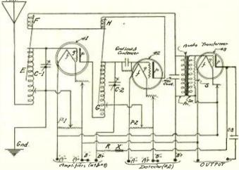
Three-tube radio-frequency receiver employing negative feedback as a stabilizer. This circuit should prove of interest to experimenters as it has many possibilities.
