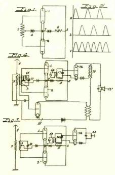
Receiver for high wave undamped reception em-bodying the heterodyne principle, but which differs in several details.
