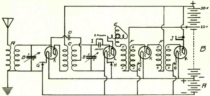
Diagram of a four-tube set embodying one stage of tuned radio-frequency, with the radio-frequency circuit neutralized. Regeneration is produced by means of the variometer in the plate lead of the second or detector tube.
