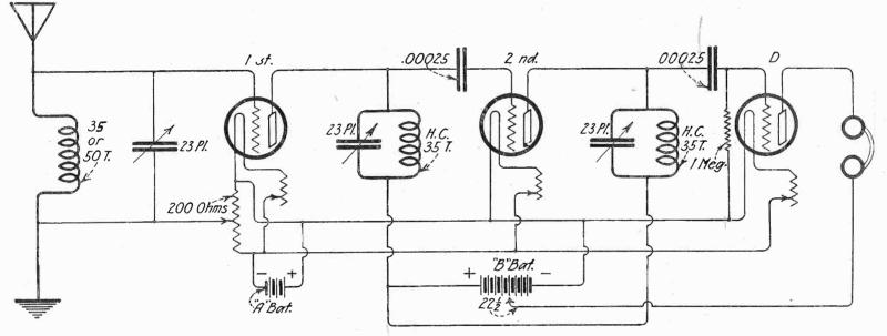
Schematic diagram of a three-tube tuned radio-frequency receiver as described in the article herewith. The constants are marked and should be followed carefully.
