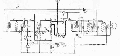
System to be used on a receiving-transmitting set designed for minimum bulk and simple control of apparatus.
