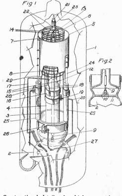
Constructional details of a high power three element tube, with special attention to the rigidity and strength of the supporting electrodes.
