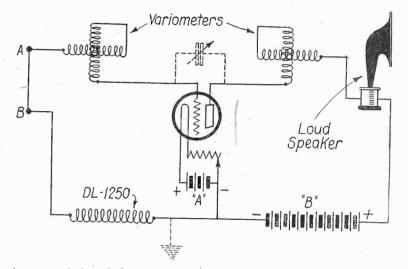
A new variation of the super principle embodying two variometers and a high value inductance coil. Tuning for wave length is accomplished by the grid variometer while the selectivity and volume is controlled by the plate variometer. Best apparatus should be used. If added selectivity is wanted, the optional condenser should be used. This condenser also permits the use of small tubes such as WD's.
