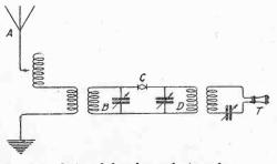
Receiver designed for the exclusion of atmospheric disturbances.
