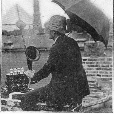
(C. International Newsreel) Berlin fan and investigator of peculiar radio phenomena, contrasting the loop antenna reception on a four tube receiver, with an antenna composed of an umbrella and his body. He holds the umbrella up, clasping its metal stem tightly, then alternately connects the loop and his own idea of an efficient antenna. The reason for his sitting atop the chimney is not stated.
