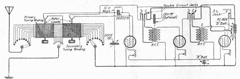
Circuit asked for by Frank Maxwell. It is the Western "duplex tuner ciruit" with two stages of audio-frequency amplification. The constants for this circuit are marked, leaving the selection of the audi-frequency transformer to the builder.
