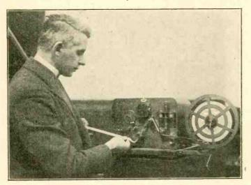
Fig. 3. Huth high-speed telegraph recorder comprising the new relay described in the accompanying article.
