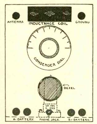
Fig. 2. Panel layout for a set embodying a single detector tube.
