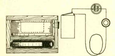
Fig. 1. Construction of a handy buzzer test and circuit diagram of connections used. A single turn of wire around the coupler or tuner is sufficient.
