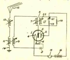
Arrangement whereby enormous self-amplifica-tion is possible on one tube.
