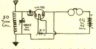
Fig. 1. Circuit diagram for the single control set. Note that the only variable feature of the set is the condenser dial, even the rheostat being done away with.
