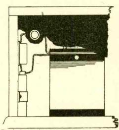
Fig. 2. Suggested method of installing a buzzer test in a cabinet set. This is the preferred method if there is room in the cabinet for the installation-
