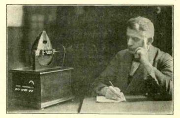
Fig. 2. A mandolin converted into a loud speaker, utilizing the principle illustrated in Fig. 1.
