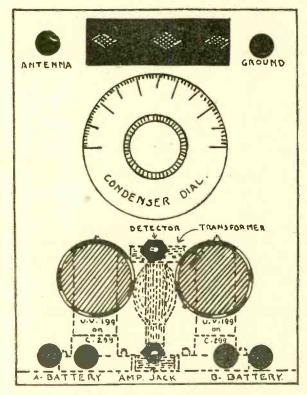
Fig. 3. Panel layout suggested for a detector and one stage set.
