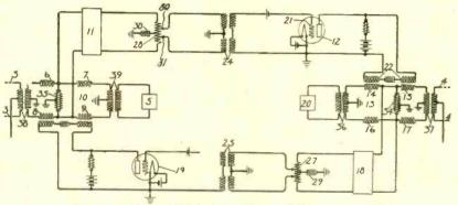
Circuit used in two-way repeater system utilizing vacuum tubes.
