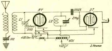
Diagram illustrating a radio-frequency set using honeycomb coils. L, primary honeycomb coil. L1, secondary honeycomb coil. L2, tuned impedance coil used as radio-frequency amplifier. The condenser shunting should be .0005 mfd.
