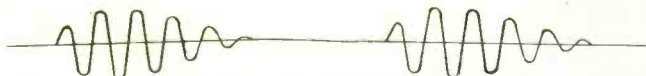
Fig. 2. Conventional method for representing a series of wave-trains sent by a transmitting station.
