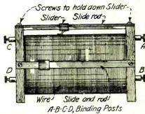
Figure 4.—A two-slide tuning coil.
