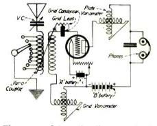
Figure 3. Schematic diagram of the wiring of the completed set. Suggested by George W. May.
