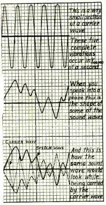
Schematic diagram showing waves.
