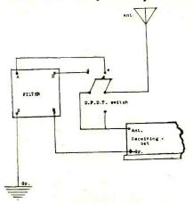
Figure 3.—Filter and receiving set connections.
