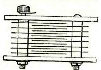
Schematic diagram showing how condenser is made.
