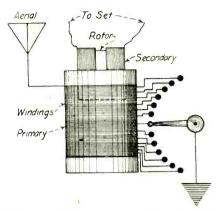
Figure 2. Detail of the method of wiring the variocoupler. Suggested by George W. May. Drawn by S. Newman.
