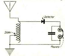
Figure 3.—Schematic diagram of a oneslide tuning coil. Suggested by George W. May. Drawn by S. Newman.
