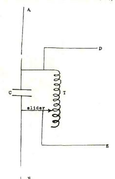
Figure 2.—A periodic filter. C, a capacity of .oo1 microfarads. T, a simple tuning coil. A, B, D, E, are terminals.
