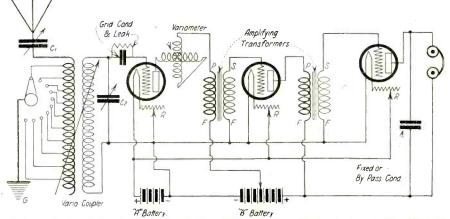
Figure 2—Schematic diagram of the wiring of the complete set. The diagram shows every part and element that is needed for the set. Suggested by H. S. Stanford. Drawn by S. Newman.
