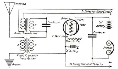
Figure 1—A one-step combined radio- and audio-frequency amplifier; but eight stages of combined amplification have been employed. Drawn by S. Newman.
