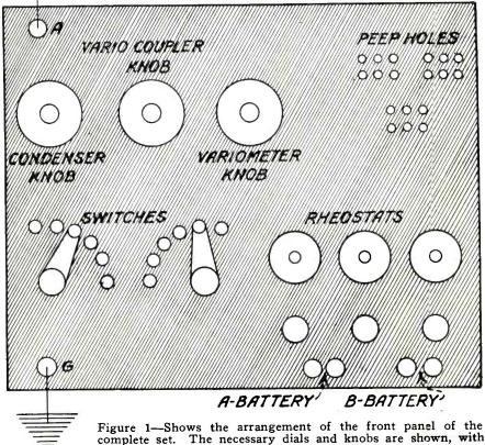
The necessary dials and knobs are shown, with rheostats and binding posts. Suggested by H. S. Stanford. Drawn by S. Newman.
