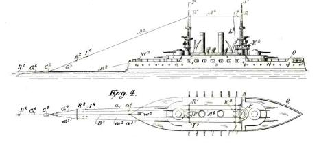
Schematic diagram explaining the invention of John Hays Hammond, Jr., for increasing the antennae of warships.
