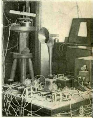
(Above) One of the most interesting new radio devices is shown in this photograph. It is called the oscillograph—a machine that either photographs currents produced in radio research work or permits the operator to watch them in action. It utilizes two distortionless amplifying tubes and two power-tubes. (C. Kadel & Herbert News Service.)
