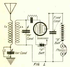
Figure 1—Schematic diagram of what is known as a straight hook-up. The various elements are shown in the circuit. Suggested by George W. May. Drawn by S. Newman.
