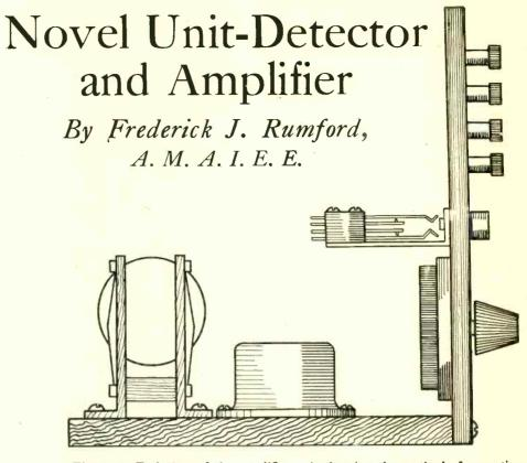
Figure 3—End view of the amplifier unit showing the method of mounting the transformer, jacks and sockets. Suggested by F. J. Rumford. Drawn by S. Newman.
