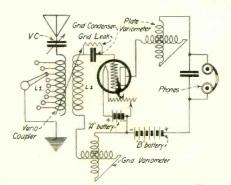
Figure 2—Schematic diagram of the socalled regenerative receiver. This is the variometer type. In the above hook-up it is easy to discern where the variometers are placed in the grid and plate circuits, respectively. Suggested by George W. May. Drawn by S. Newman.
