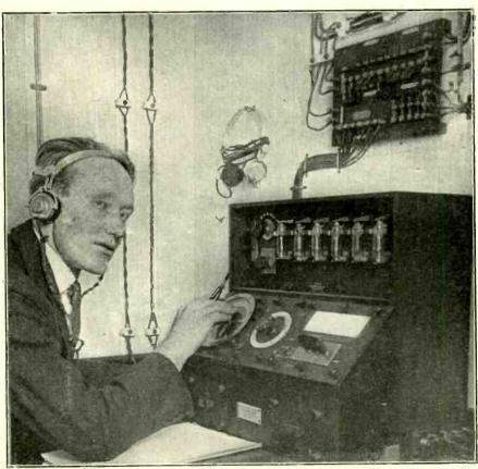
(Above) The latest type of Marconi direction finder—an aerial of two loops at right angles to each other—which determines the direction of messages from shore stations and ascertains the exact location of a ship in a fog. The instrument is one of the new wonders in radio. (C. Ewing Galloway, N. Y.)
